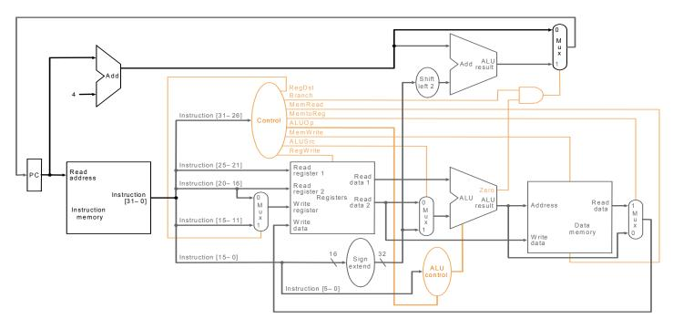
The figure above shows the basic datapath you will implement. The control logic has been highlighted. Below is an abbreviated truth table for the Control unit. Assume the op codes are 000000, 100011, 101011, and 000100 for R-format, lw, sw and beq respectively.
