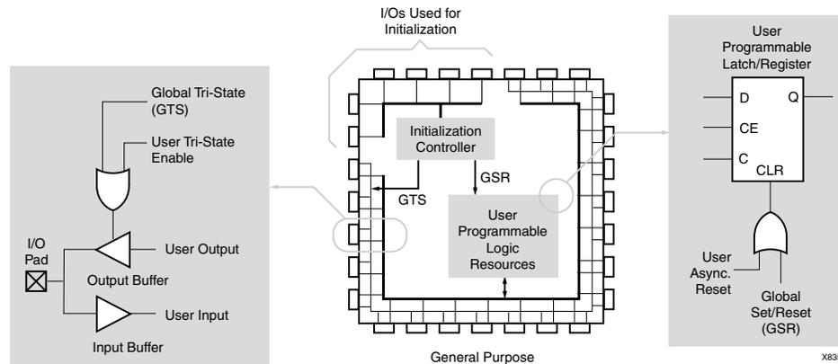
Figure 6-1: Built-in FPGA Initialization Circuitry Diagram
