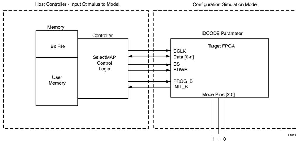
Figure 6-2: Block Diagram of Model Interaction
