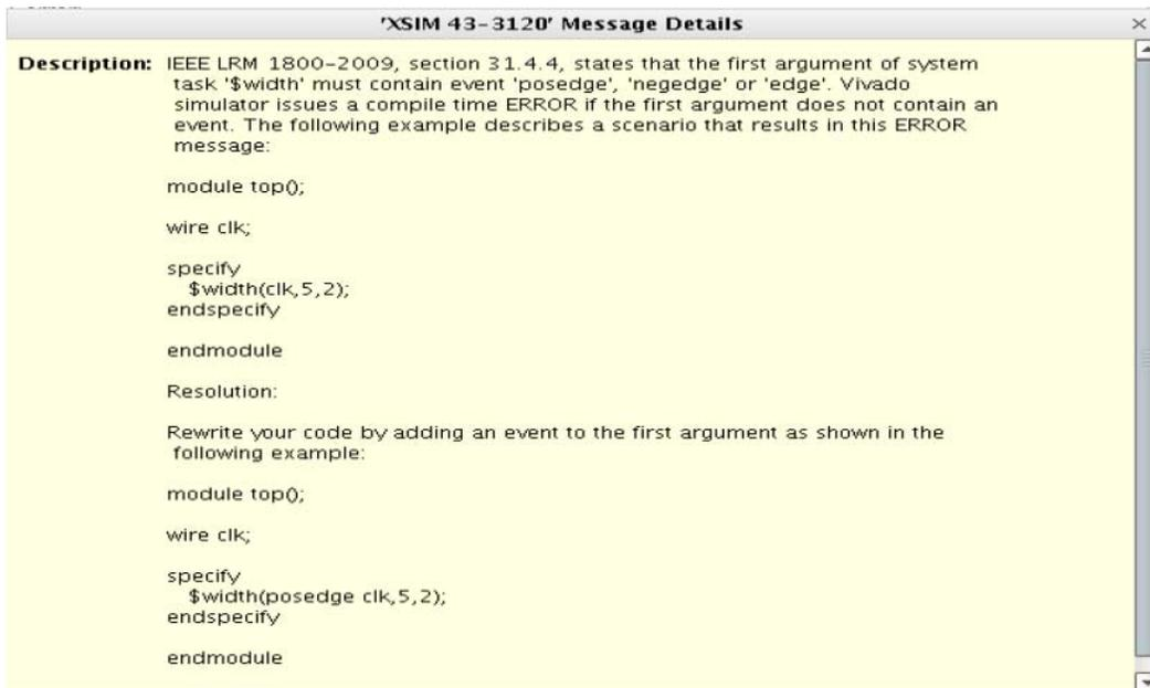
Figure 3-16: Simulator Message Description and Resolution Information
