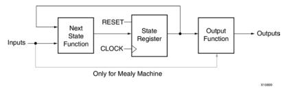
For a Hardware Description Language (HDL), *process* (VHDL) and *always blocks* (Verilog) are the best ways to describe FSM components. Xilinx® uses *process* to refer to both VHDL *processes* and Verilog *always blocks*.
