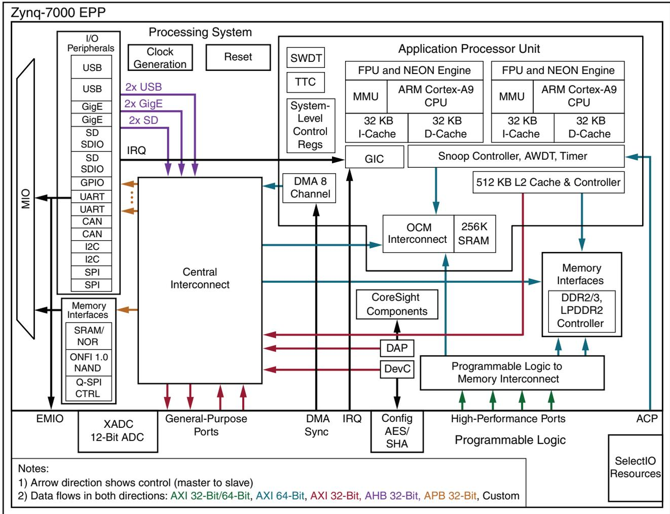
Figure 2-1: Zynq-7000 AP SoC Processor System High-Level Diagram
