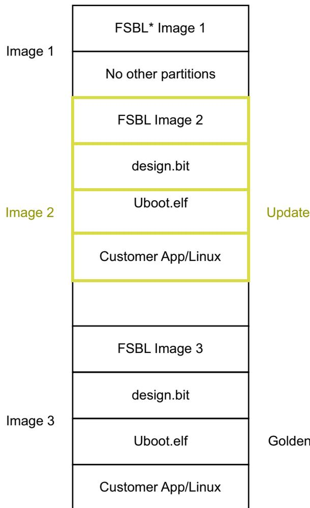
Figure 3-13: Flash Partitions for Secure Boot with eFUSE
