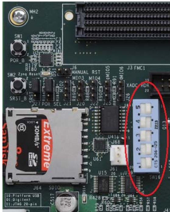
Figure 5-6: Jumper Settings for Booting Linux from SD Card
