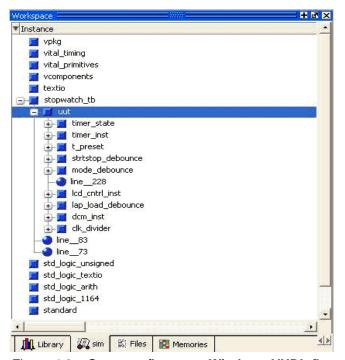
Figure 4-3: Structure/Instance Window - VHDL flow
