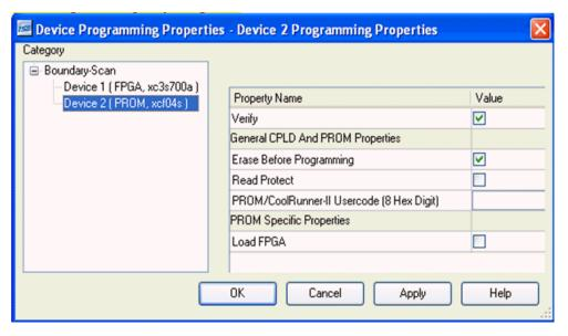
Figure 7-8: Program Options for XC3S700A Device
