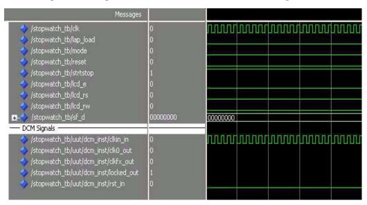
Figure 4-4: Waveform After Adding DCM Signals Divider
