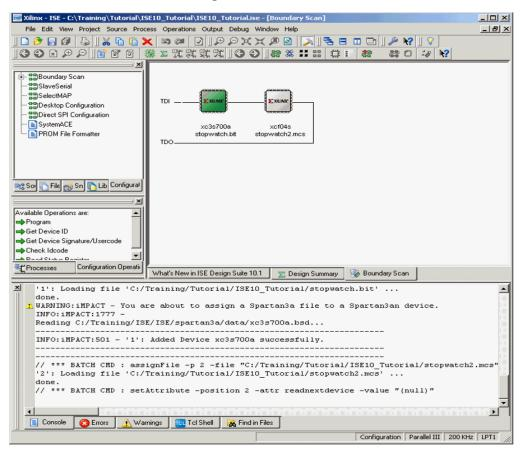
Figure 7-6: Available Boundary Scan Operations for an XC3S700A Device
