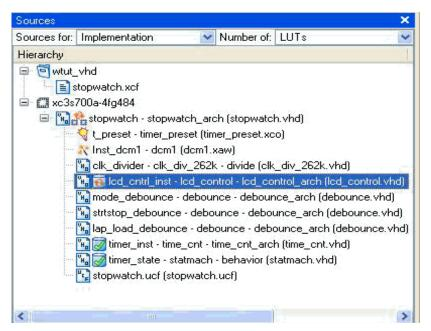
Figure 5-28: LCD\_CNTRL\_INST Partition is Out of Date
