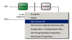
Figure 7-13: Selecting a Boundary Scan Operation
