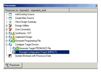
Figure 7-1: Opening iMPACT from ISE
