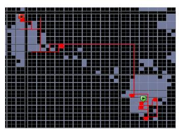
Figure 5-26: Floorplan Implemented - Data Path with Simplified Routing
