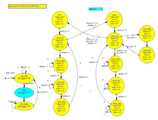
Figure 3-19: Incomplete State Machine Diagram
