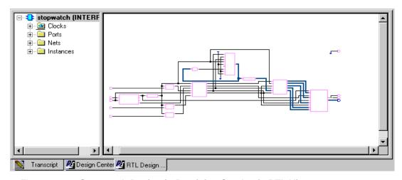
Figure 2-23: Stopwatch Design in Precision Synthesis RTL Viewer
