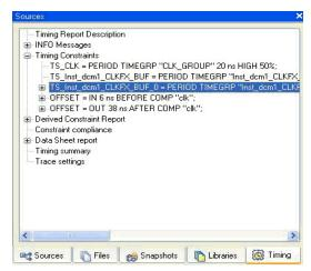
Figure 5-21: Selecting Post-Map Static Timing constraint
