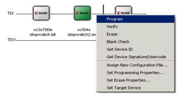
Figure 7-15: Available Boundary Scan Operations for a XCF02S Device
