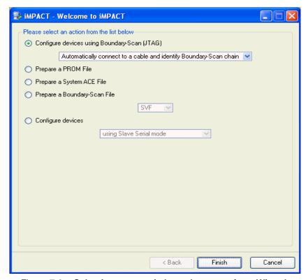
Figure 7-3: Selecting automatic boundary scan from Wizard
