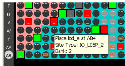
Figure 5-13: Assigning I/O Pins by Dragging into Package View
