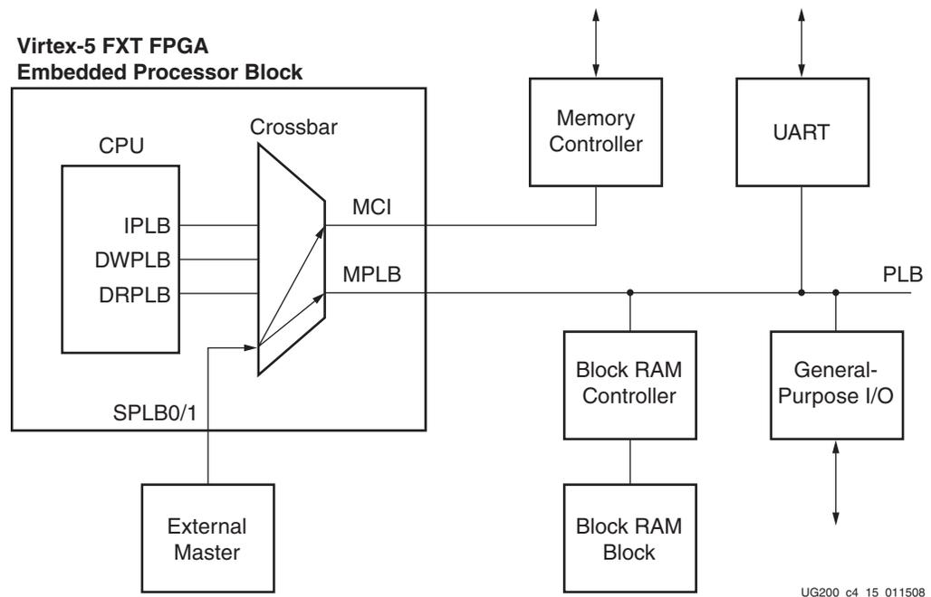
Figure 4-15: Main Memory and Peripherals Shared Between Processor and External Master
