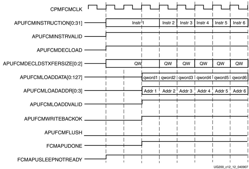
**Figure 12-12: Quadword Load Back-to-Back Instructions (3:1 Clock Ratio or Higher)**
