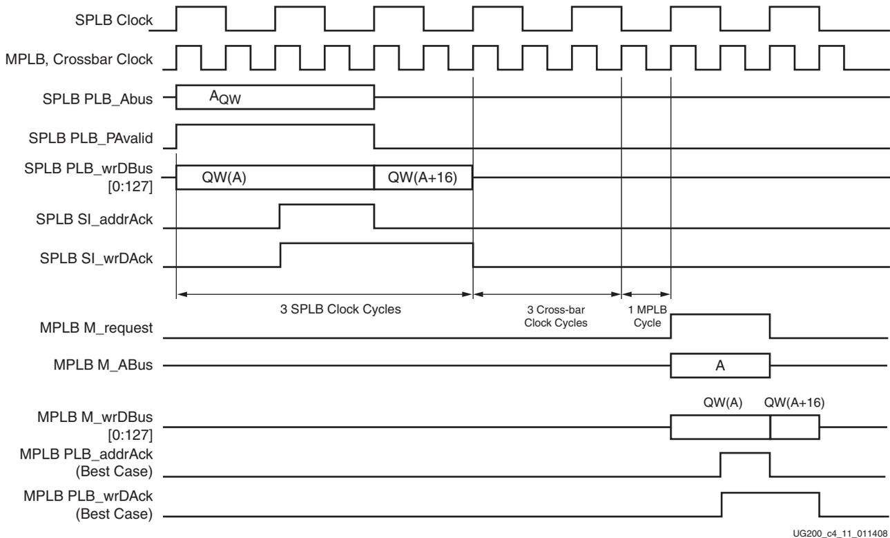
Figure 4-11: SPLB to MPLB 2-Quadword Burst Write with 1:2 Clock Ratio
