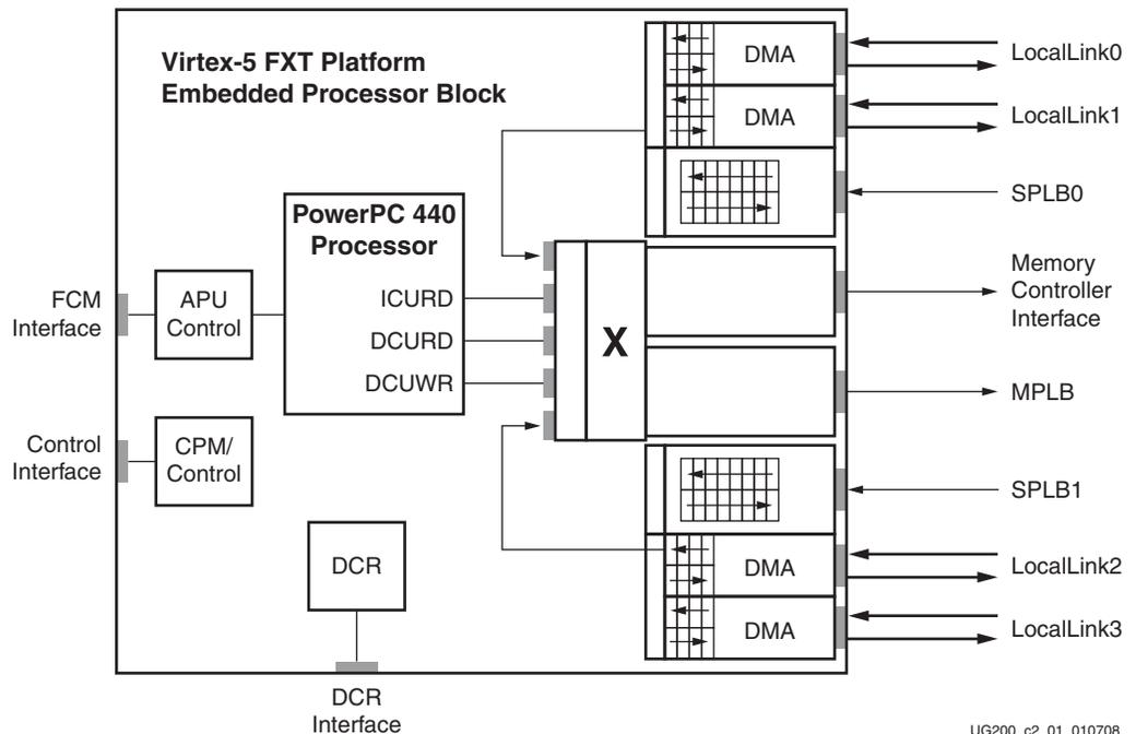
Figure 2-1: Embedded Processor Block in Virtex-5 FPGAs
