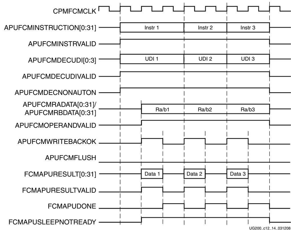
**Figure 12-14: Non-Autonomous Instructions with Early Confirm Back-to-Back (2:1 Clock Ratio or Higher)**
