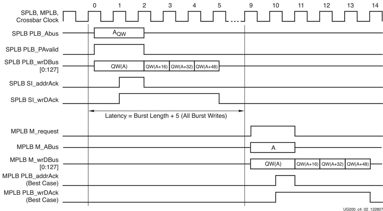
Figure 4-2: SPLB to MPLB 4-Quadword Burst Write Transaction
