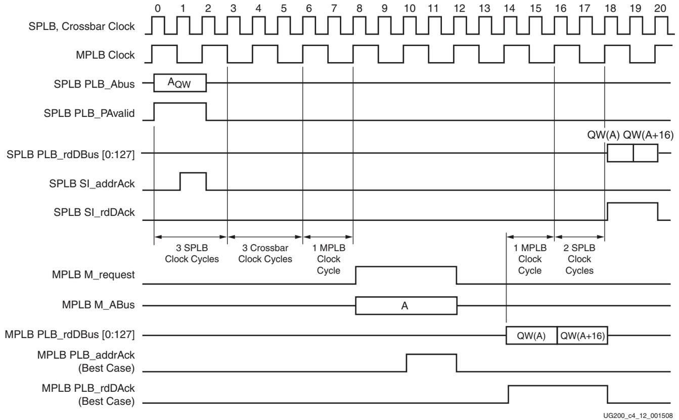
Figure 4-12: SPLB to MPLB 2-Quadword Burst Read with 2:1 Clock Ratio
