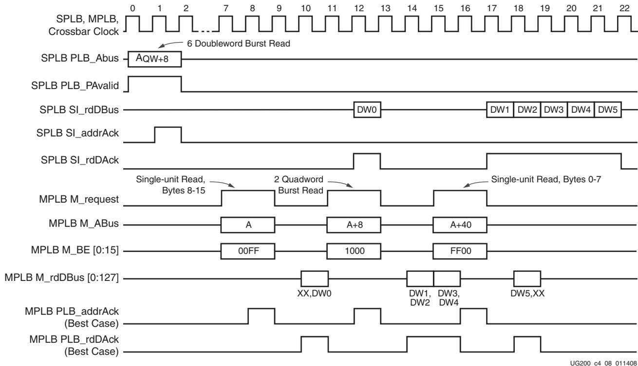
Figure 4-8: SPLB to MPLB 6-Doubleword Unaligned Burst Read from 128-Bit Slave (Requested by a 64-Bit Master)
