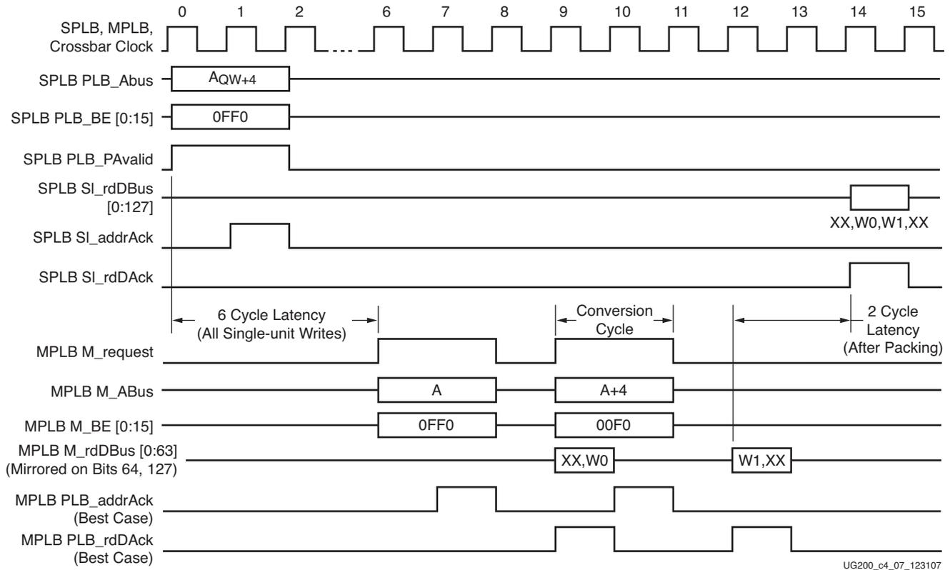
Figure 4-7: SPLB to MPLB Single-Unit Read of 2 Unaligned Words by 128-Bit Master from 64-Bit Slave
