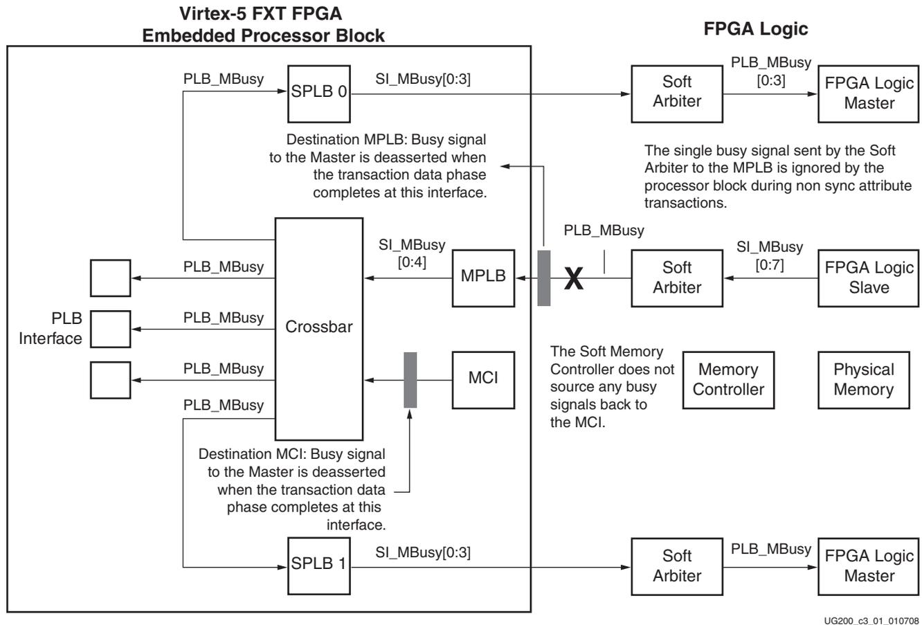
Figure 3-1: Busy Signals in FPGA Logic and Embedded Processor Block
