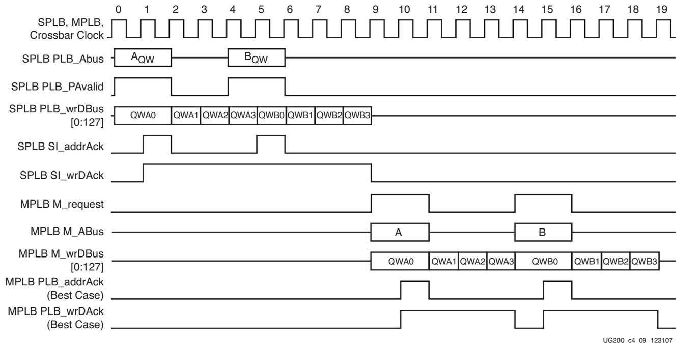
Figure 4-9: SPLB to MPLB Back-to-Back 4-Quadword Burst Writes Between 128-Bit Devices
