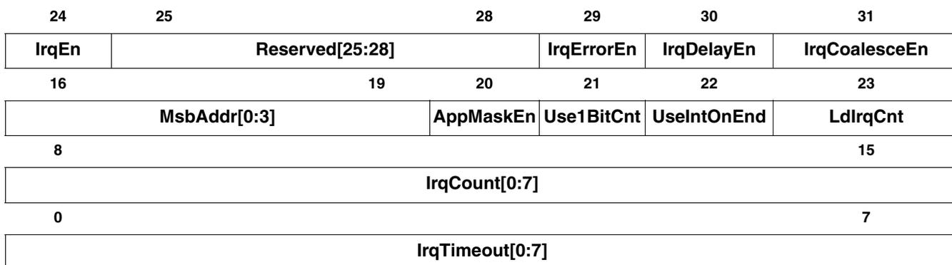
Figure 13-26: RX Channel Control Register
