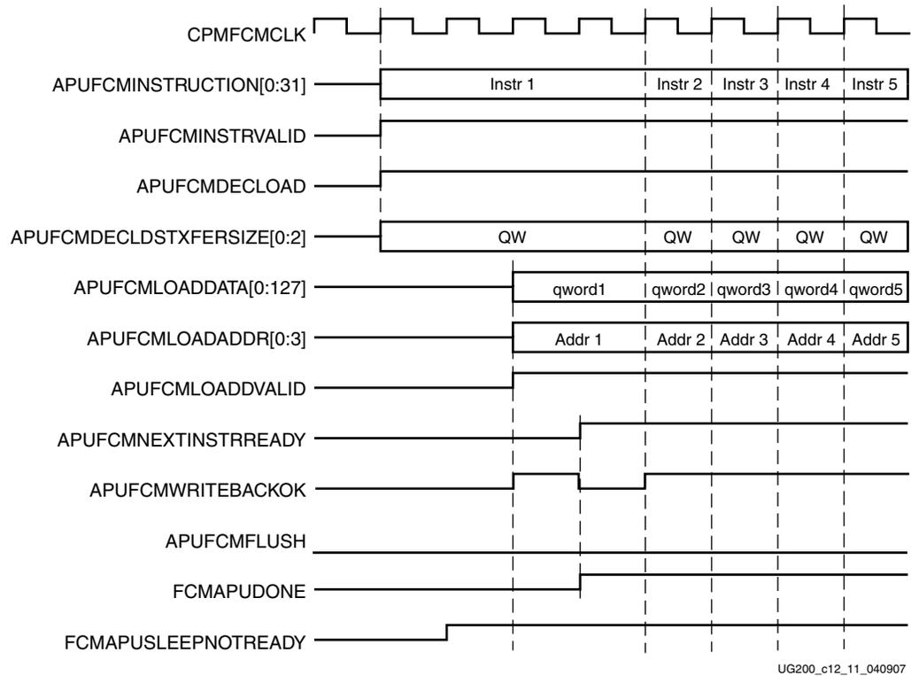
Figure 12-11: Quadword Load Back-to-Back Instructions (4:1 Clock Ratio or Higher)
