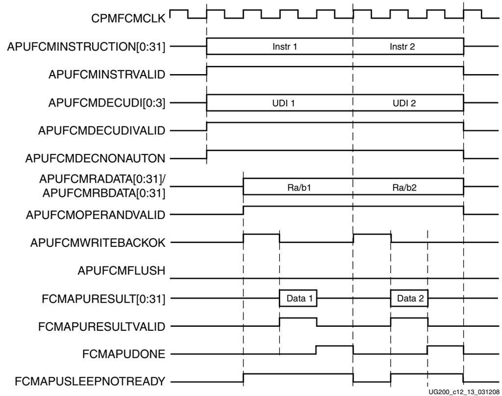
Figure 12-13: Non-Autonomous Instructions with Early Confirm Back-to-Back (3:1 Clock Ratio or Higher)
