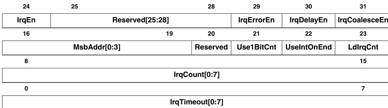
Figure 14-10: TX Channel Control Register
