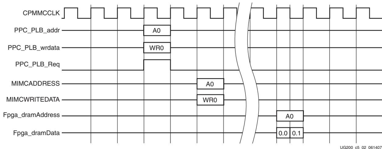
Figure 5-2: System-Level Timing Diagram: Write
