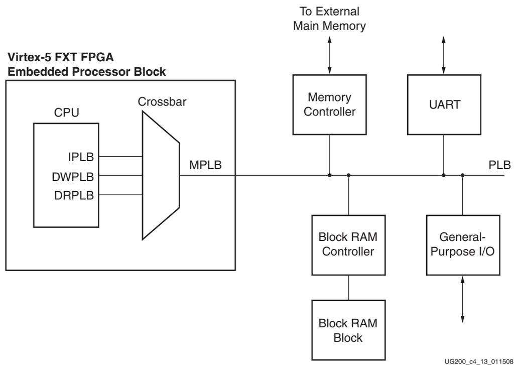
Figure 4-13: Simple Processor-Centric Shared Bus Design
