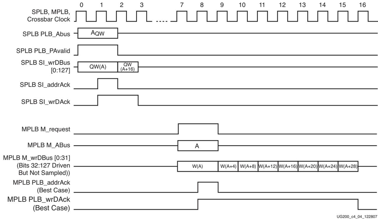
Figure 4-4: SPLB to MPLB 2-Quadword Burst Write by 128-Bit Master to 32-Bit Slave
