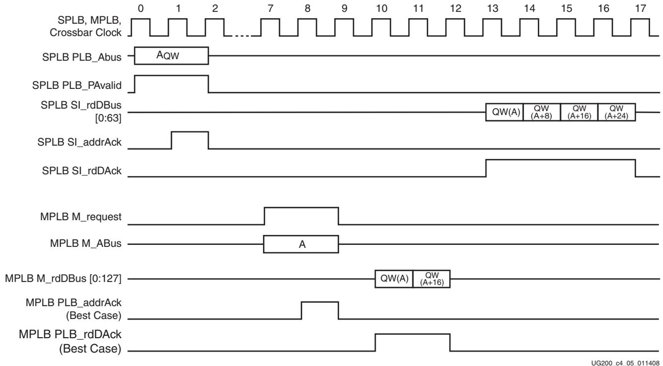
Figure 4-5: SPLB to MPLB 4-Doubleword Burst Read by 64-Bit Master from 128-Bit Slave (Aligned)
