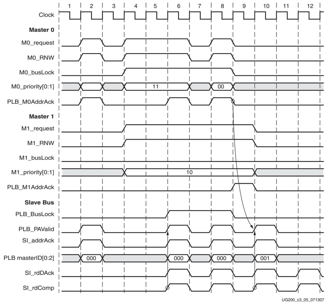
Figure 3-5: Locked Transfer Waveforms
