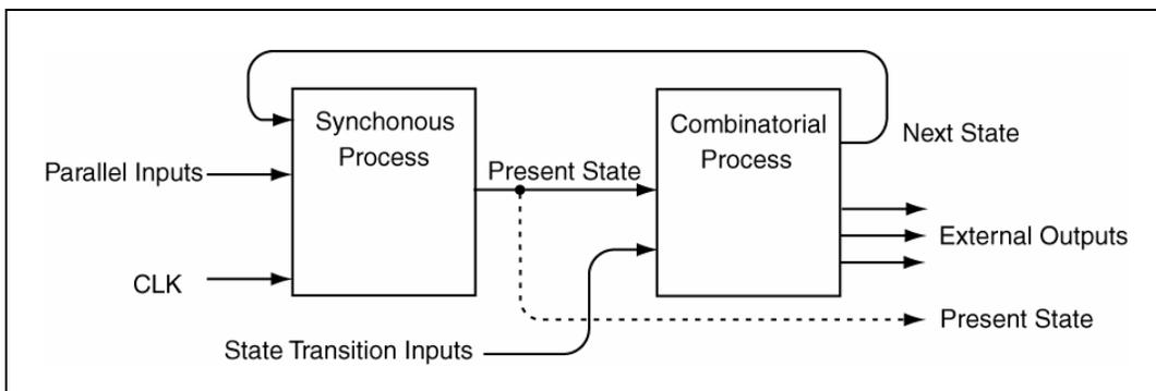
**Figure 47: Model for VHDL implementations of FSMs.**
