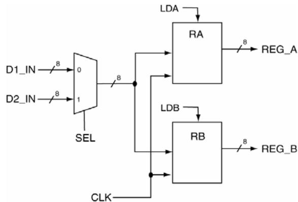
**Solution:** The circuit shown in EXAMPLE 30 includes two 8-bit registers and a 2:1 MUX. This is an example of a bus-based data transfer in the output of the MUX is connected to the inputs of the two registers. Each of the two registers has their own independent load control input. The solution to EXAMPLE 31 is shown in Figure 67. And as we've grown to expect, there are a couple of things worth noting about this solution.
