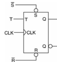
7. Provide a VHDL behavioral model of the T flip-flop shown at the right. The S and R inputs are an active high asynchronous preset and clear. Assume both the S and R inputs will never be asserted simultaneously.
