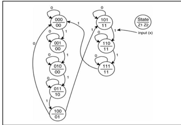
8. Write a VHDL behavioral model that could be used to implement the state diagram on shown in the right. The state variables should be encoded as listed and also provided as outputs of the FSM.
