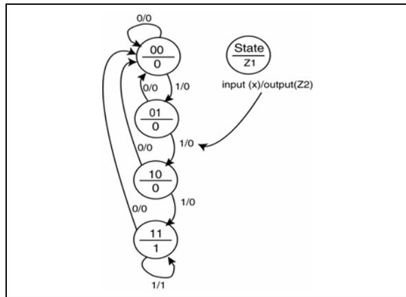
9. Write a VHDL behavioral model that could be used to implement the state diagram on shown in the right. The state variables should be encoded as listed and also provided as outputs of the FSM.
