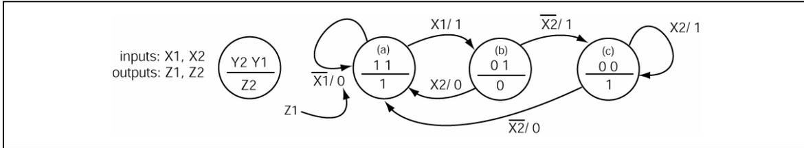
12. Write a VHDL behavioral model that could be used to implement the state diagram on shown in the right. The state variables should be encoded as listed and also provided as outputs of the FSM.
