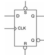
5. Provide a VHDL behavioral model of the T flip-flop shown on the right. The S and R inputs are an active low asynchronous preset and clear. Assume both the S and R inputs will never be asserted simultaneously. Implement this flip-flop first using an equation description of the outputs and then using a behavioral description of the outputs.
