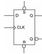
2. Provide a VHDL behavioral model of the D flip-flop shown on the right. The S and R inputs are an active low asynchronous preset and clear. Assume the S input takes precedence over the R input in the case where both are asserted simultaneously.
