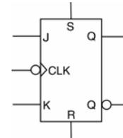
9. Provide a VHDL behavioral model of the JK flip-flop shown on the right. The S and R inputs are an active low asynchronous preset and clear. Assume both the S and R inputs will never be asserted simultaneously.
