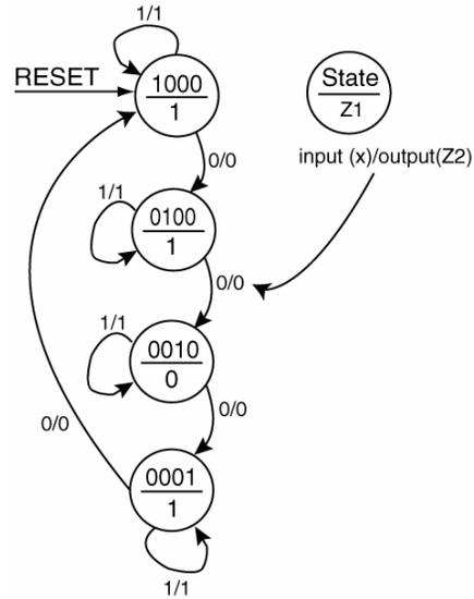
**Solution:** The state diagram shows four states, one external input X, two external outputs Z1 and Z2 with the Z2 output being a Mealy output. This is a Mealy machine that indicates one-hot encoding should be used to encode the state variables. We'll approach this solution in pieces, bits and pieces.
