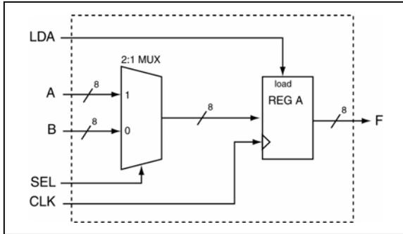
2. Provide a VHDL model that can be used to implement the following circuit.
