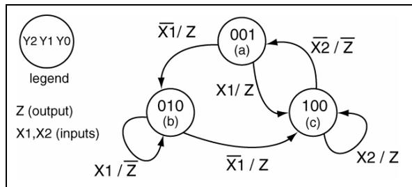
11. Write a VHDL behavioral model that could be used to implement the state diagram on shown in the right. The state variables should be encoded as listed and also provided as outputs of the FSM.
