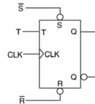
6. Provide a VHDL behavioral model of the T flip-flop shown on the right. The S and R inputs are an active low asynchronous preset and clear. Assume both the S and R inputs will never be asserted simultaneously.
