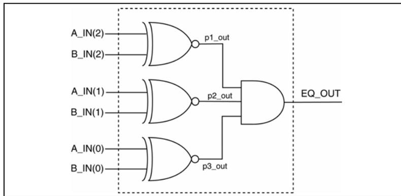
**Figure 60: Discrete gate implementation of a 3-bit comparator.**
