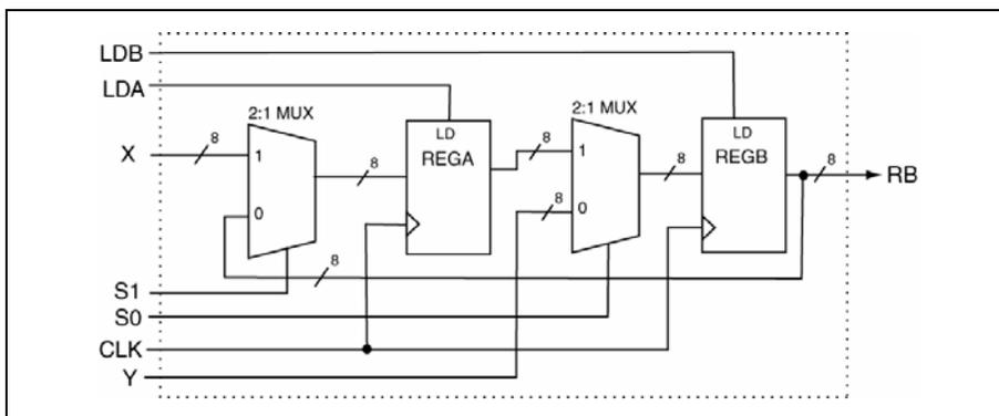
4. Provide a VHDL model that can be used to implement the following circuit.
