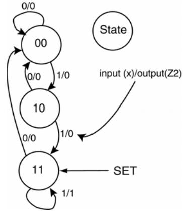
**Solution:** The state diagram shown in the problem description indicates that this is a three-state FSM with one Mealy-type external output and one external input. Since there are three states, the solution requires at least two state variables to handle the three states. The black box diagram of the solution is shown in Figure 52. Note that the two state variables are handled as a bundled signal.
