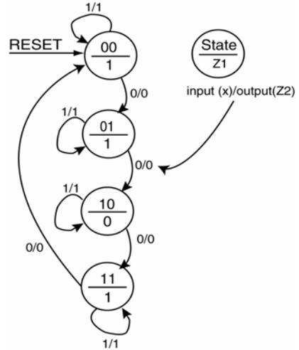
**Solution:** The state diagram indicates that the solution will contain four states, one external input, and two external outputs. This is a hybrid FSM in that the *if* contains both a Mealy and Moore-type output but in this case, the FSM would be considered a Mealy-type FSM. The black box diagram for the solution is shown in Figure 54 and the actual solution is shown in Figure 55.
