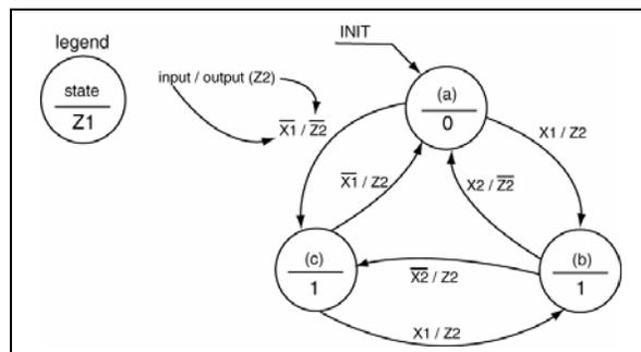
Draw the state diagram associated with the following VHDL code. Consider the outputs Y to be representative of the state variables. Be sure to provide a legend. Indicate the states with both the state variables and their symbolic equivalents.
