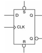
3. Provide a VHDL behavioral model of the D flip-flop shown on the right. The S and R inputs are synchronous preset and clear. Assume both the S and R inputs will never be asserted simultaneously.
