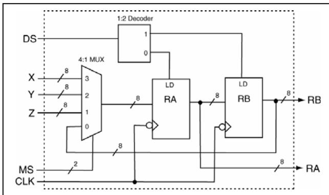
3. Provide a VHDL model that can be used to implement the following circuit.
