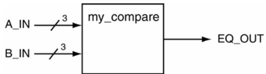
**Solution:** A comparator is one of the classic combinational circuits that every digital design student must derive at some point in their careers. The solution presented here implements the discrete gate version of the circuit which is shown in Figure 60. Once again, the solution presented here is primarily an example of a VHDL structural model and does not represent the most efficient method to represent a comparator using VHDL.
