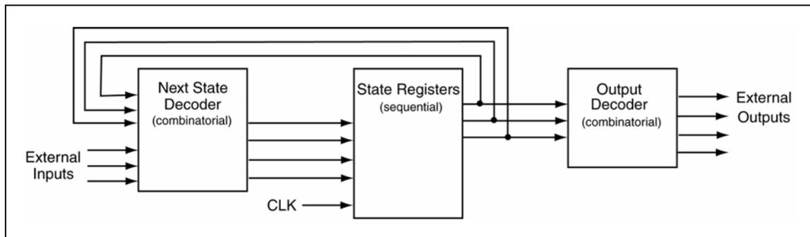
**Figure 46: Block diagram for a Moore-type FSM.**
