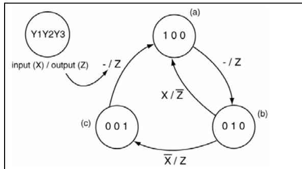
10. Write a VHDL behavioral model that could be used to implement the state diagram on shown in the right. The state variables should be encoded as listed and also provided as outputs of the FSM.
