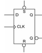
4. Provide a VHDL behavioral model of the D flip-flop shown on the right. The S and R inputs are an active low asynchronous preset and clear. If both the S and R inputs are asserted simultaneously, the output of the flip-flop will toggle.
