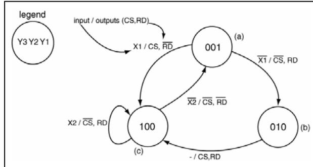
13. Write a VHDL behavioral model that could be used to implement the state diagram on shown in the right. The state variables should be encoded as listed and also provided as outputs of the FSM.
