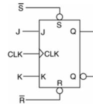
10. Provide a VHDL behavioral model of the JK flip-flop shown on the right. The S and R inputs are active low synchronous preset and clear. Assume both the S and R inputs will never be asserted simultaneously.
