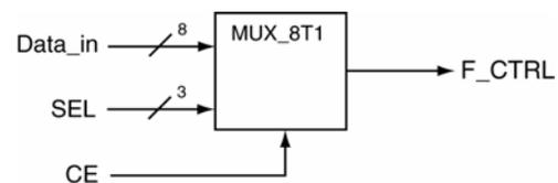
**Solution:** This solution to *EXAMPLE 13* is shown in Figure 40. The entity declaration is repeated below for your convenience. This solution places the *case* statement in the body of an *if* construct. In case you've not noticed it yet, the number of possible solutions to a given problem increases as the circuits you're implementing become more complex.
