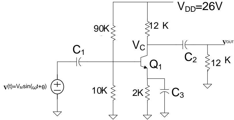
2. Determine the small signal output voltage if the small signal input voltage is a sinusoidal 1 KHz signal with 0-P amplitude of 10mV.
