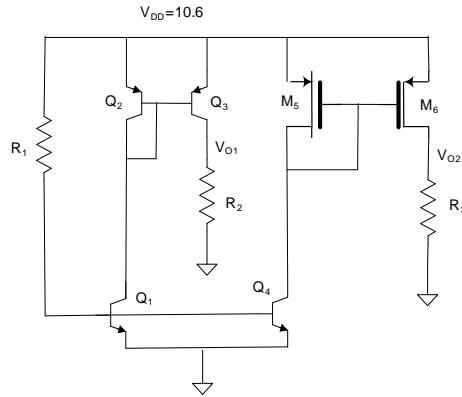
5. Assume the biasing voltages have been selected so that the quiescent current is 1 mA and that all transistors are operating in the forward active region. Determine the small-signal voltage gain and  $R_o$  for the following two circuits. Assume  $\beta = 100$  and  $V_{AF} = 130V$  for all transistors.
