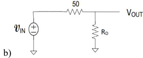
c.) Treat Diode as a box with  $V_d$  as one terminal and  $I_d$  as another, we know that  $V_D = V_t * \ln\left(\frac{I_{DQ}}{J_s A_D}\right)$
