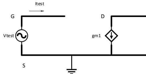
There is no current flowing in the input terminal (due to the open circuit).  $R_{in} = \infty$
