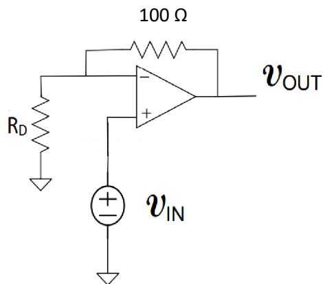
$$R_D = \frac{V_t}{I_{DQ}} = \frac{25.85mV}{1mA} = 25.85 \Omega$$
