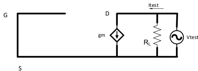
$$\text{Since } V_{in} = 0, V_T = I_T * R_L \rightarrow R_{out} = \frac{V_T}{I_T} = R_L$$
