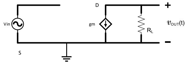
Note that the output resistance was simplified  $\frac{1}{g_0} || R_L \approx R_L$
