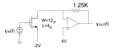
**Problem 7** Consider the following circuit operating at T=300K. Assume  $V_{IN}$  is a small-signal voltage source.
