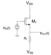
**Problem 4** Consider the following circuit where R1=20K. Size the device so that the amplifier has a voltage gain of -10. Assume  $M_1$  is in saturation.
