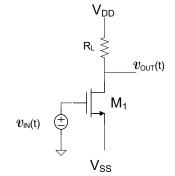
a) Draw the small signal equivalent circuit (showing  $g_m$  and  $g_0$ ), and solve for the small signal gain.
