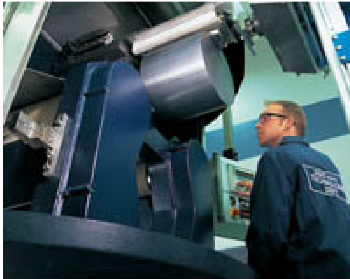
A section of 300mm ingot is loaded into a wiresaw
