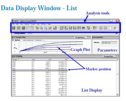
The List Display corresponds exactly with the Graph Plot. Even the highlighted line of data corresponds to the marker position on the Graph Plot.
