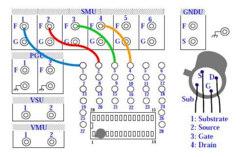
For all class exercises, you need the 28-pin dual in line socket which comes standard with the 4145 fixture (16058A) or the newer fixture (16442A/B). Either fixture works fine.
