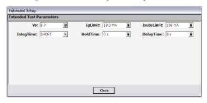
The Extended Setup dialog box allows the user to set the additional test setup parameters. In the Id-Vd setup, the additional parameters are source voltage, maximum gate current, maximum substrate current, integration time, hold time, and delay time.
