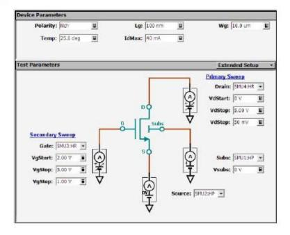
Recall Id-Vd application test setup data.
