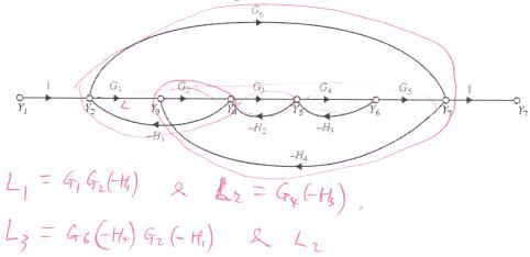
11. In the signal flow graph of problem 10, draw the remaining signal flow graph after we have removed the forward path involving G6. Find the determinant D for the graph.
