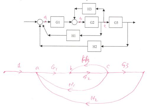
9. Find the input output transfer function for the system in problem 8.
