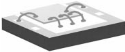
Fig. 9. Wire-bonding illustration of the LLP package.
