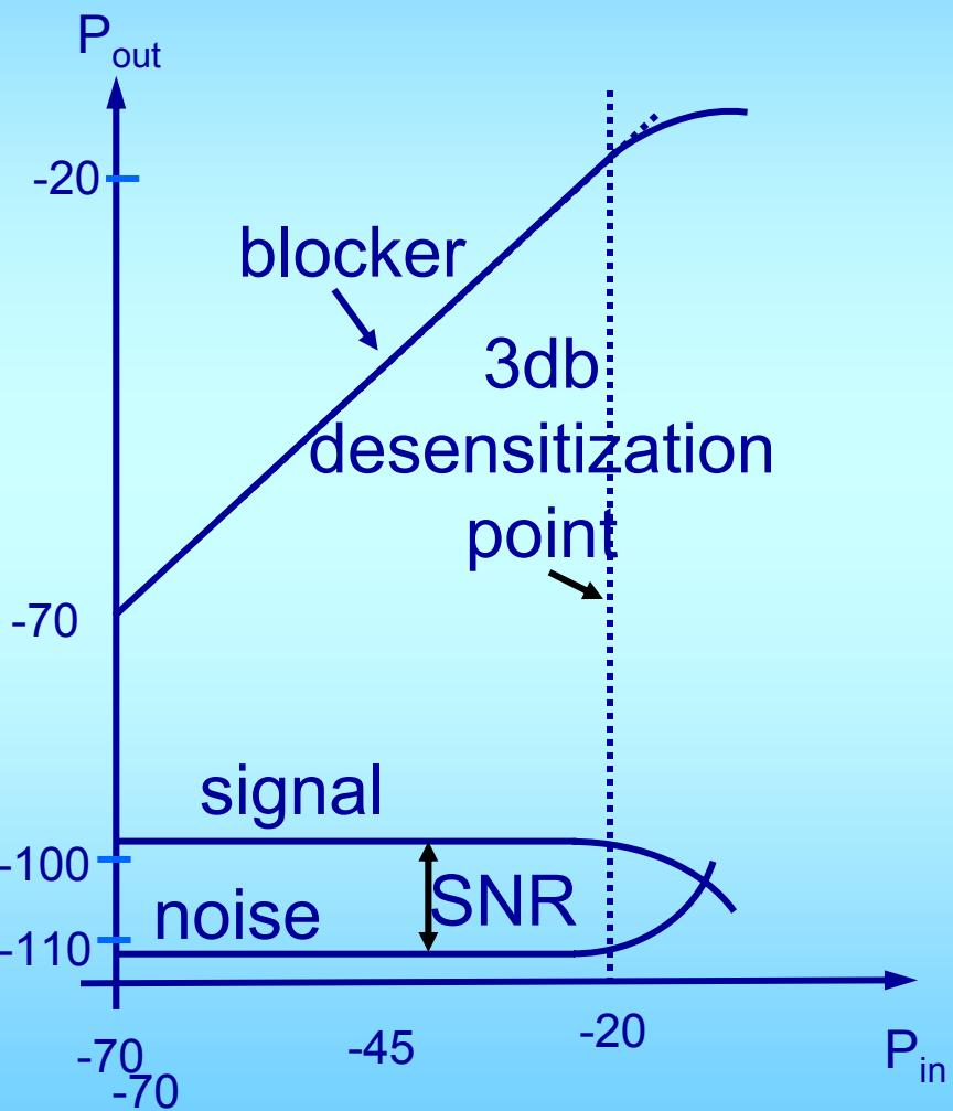
As block power become excessive, signal gain is reduced, equivalent noise is increase.
