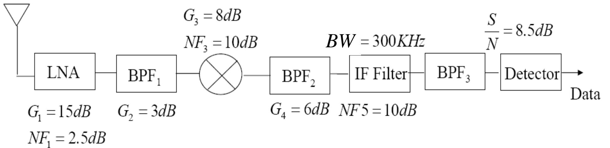
$$F_{tot} = F_1 + \frac{F_2 - 1}{G_1} + \frac{F_3 - 1}{G_1 G_2} + \frac{F_4 - 1}{G_1 G_2 G_3} + \frac{F_5 - 1}{G_1 G_2 G_3 G_4} = 2.42 = 3.8dB$$
