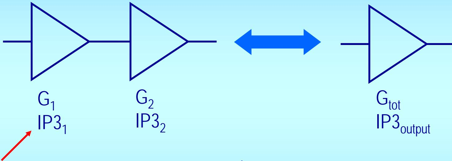
$$IP3_{\text{output}} = \frac{1}{\sum_i \frac{1}{IP3_i G_{i+1}^2 G_{i+2}^2 \cdots G_n^2}} (mW)$$
