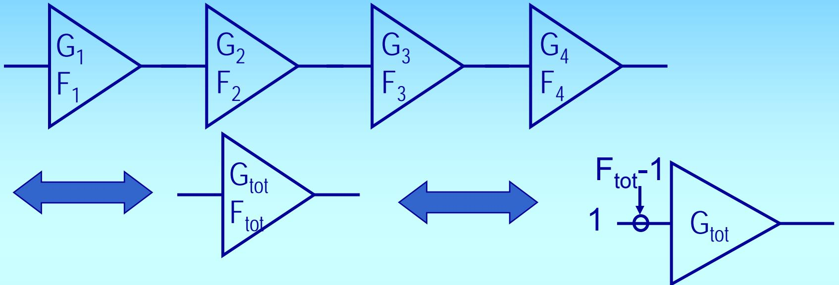
$$F_{tot} = 1 + \frac{F_1 - 1}{1} + \frac{F_2 - 1}{G_1} + \frac{F_3 - 1}{G_1 G_2} + \frac{F_4 - 1}{G_1 G_2 G_3} + \dots$$
