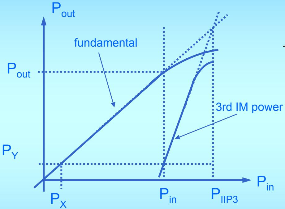
$$\begin{aligned}P_{IIP3} &= P_{in} + \frac{P_{out} - P_Y}{2} \\&= P_{in} + \frac{(P_{in} + G) - (P_X + G)}{2} \\&= \frac{3P_{in} - P_X}{2} \\P_{in} &= \frac{2P_{IIP3} + P_X}{3}\end{aligned}$$
