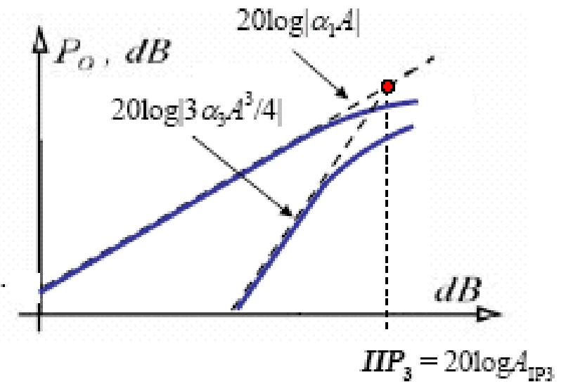
For small amplitudes the fundamental rises linearly with  $A$ , and the 3rd order intermodulation terms with  $A^3$
