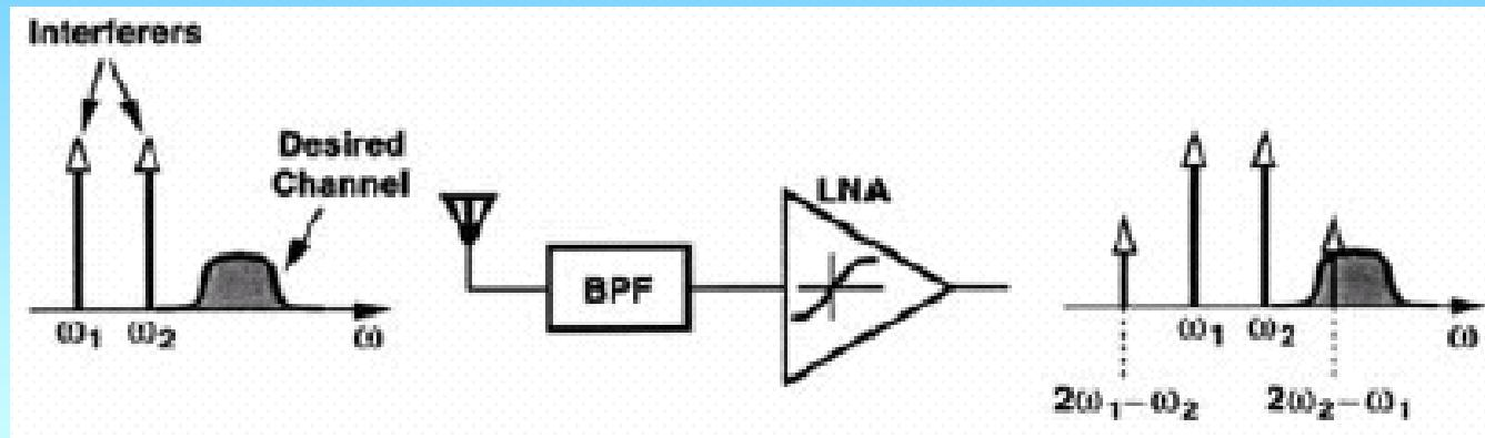
Corruption of a signal due to intermodulation
