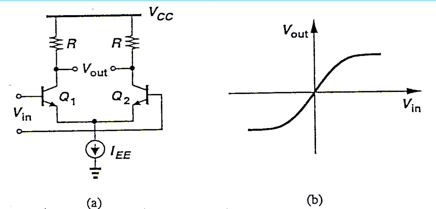
$$V_{out} = RI_{EE} \tanh \frac{V_{in}}{2V_T}$$
