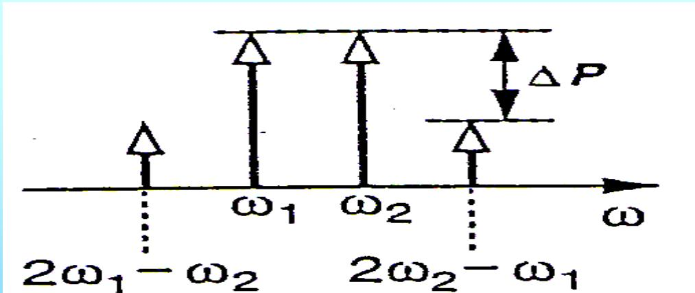
$$IP_3|_{\text{dBm}} = \frac{\Delta P|_{\text{dB}}}{2} + P_{in}|_{\text{dBm}}$$
