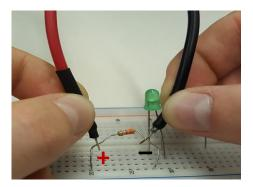
Note: This student could have put the cables into the breadboard, as well. If you choose to do this, make sure the cable is a breadboard socket in the same row as the corresponding resistor pin. See image below for reference:
