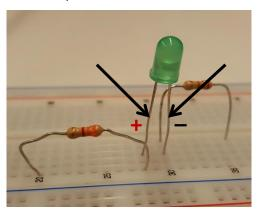
**Note:** Unless specified in the lab, you can choose which of the two points will be the positive (+) and negative (-) points. Just make sure you take note of your choice when recording your voltage measurement. Indeed, the voltage value will depend on which way you choose!
