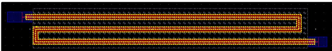
Figure 1: Resistor layout utilizing serpentine poly, metal interconnects, and *res\_id*.
