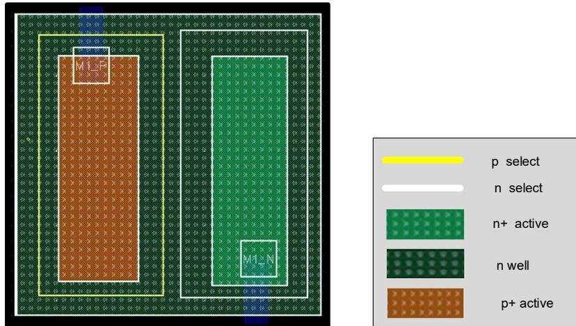
Figure 3: Simple P+ Diode Layout, Cross-sectional View
