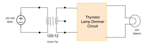
You should be able to continuously adjust the brightness of the bulb from no light output to full intensity. Since you are not controlling a large amount of current, the thyristors that have been specified for this experiment can operate safely without adding a heat sink. But be sure not to touch these devices when operating or immediately after turning off the power as they may be hot.
