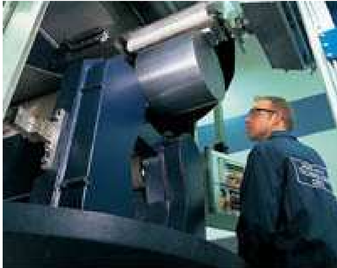
A section of 300mm ingot is loaded into a wire saw
