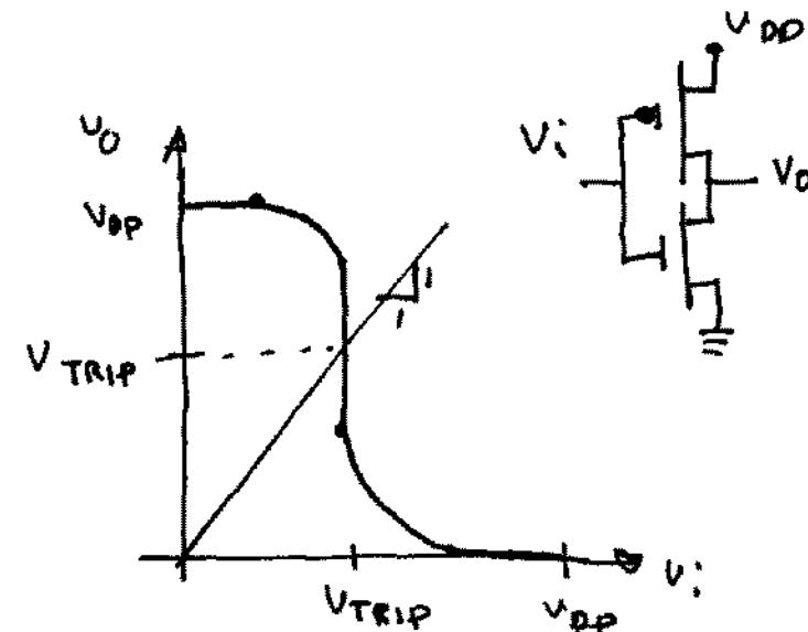
$$V_{TRIP} = \frac{.2V_{DD} + (V_{DD} - .2V_{DD})V}{1 + V}$$
