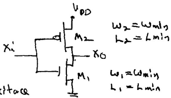
Define  $C^*$  to be the input capacitance to this inverter.  $\therefore$
