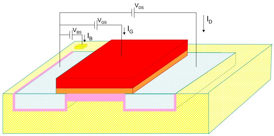
Increase  $V_{GS}$ ( $V_{DS}$  and  $V_{BS}$  assumed to be small) Depletion region in channel becomes larger
