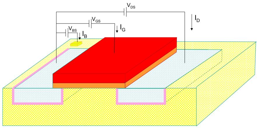
$\begin{array}{l} \mbox{Apply small } V_{GS} \\ (V_{DS} \mbox{ and } V_{BS} \mbox{ assumed to be small}) \\ \mbox{Depletion region at drain and source block current} \\ \mbox{Termed "cutoff" region of operation} \end{array}$
