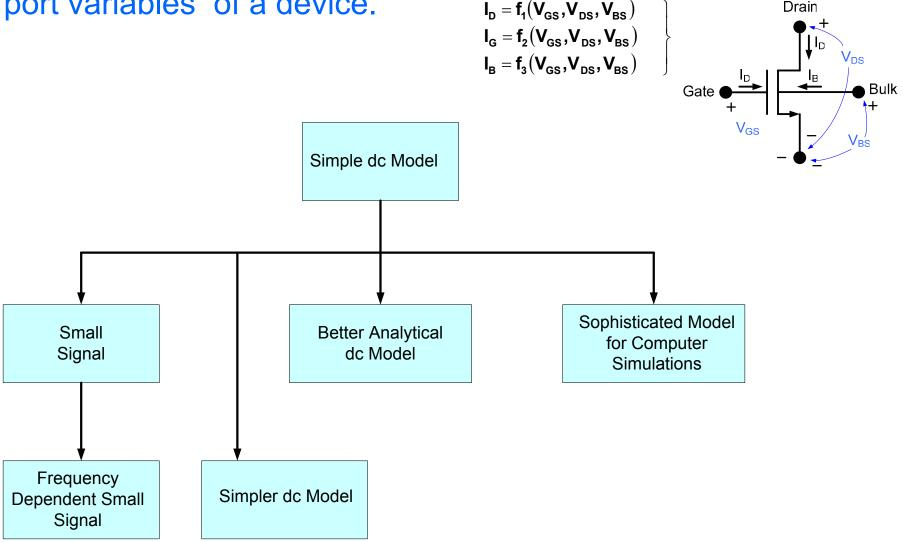
Goal: Obtain a mathematical relationship between the port variables of a device.  $I_{D} = f_{1}(V_{GS}, V_{DS}, V_{BS})$
