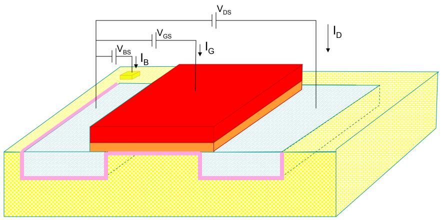
Apply small  $V_{GS}$  but a little larger than before ( $V_{DS}$  and  $V_{BS}$  assumed to be small) Depletion region electrically induced in channel Termed "cutoff" region of operation
