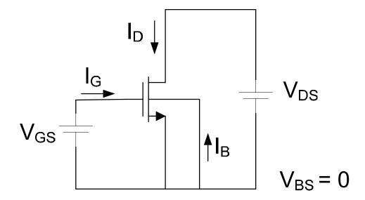
For V<sub>DS</sub> small  $R_{CH} = \frac{L}{W} (V_{GS} - V_{T})^{-1} \frac{1}{\mu C_{OX}}$
