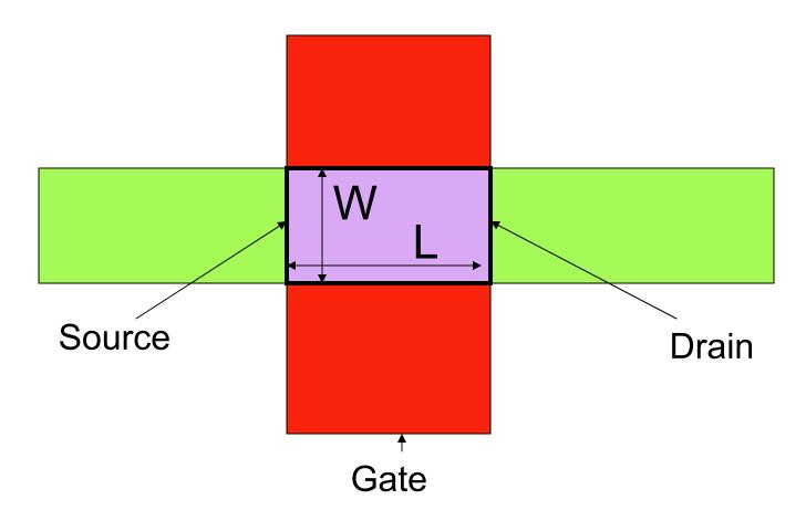
Actual Drain and Source at Edges of Channel
