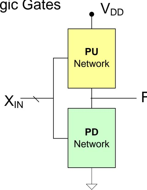
Implement  $\bar{F}$  in PD Network with n-channel devices
