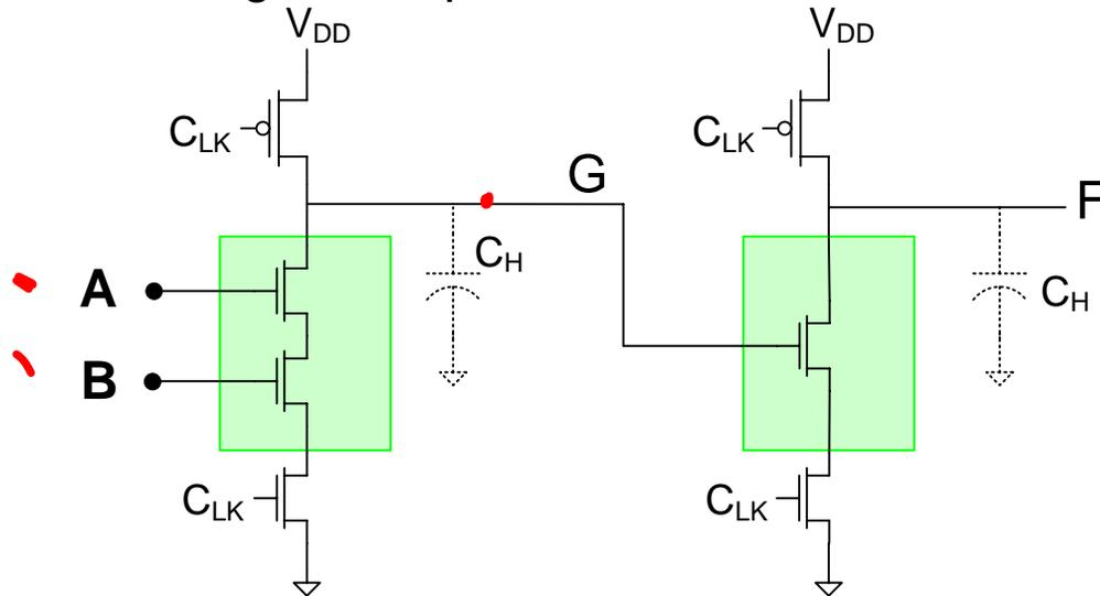
When G is precharged high and is to go Low ( $A=B=1$ ) on the evaluate state F should be a 1 but may be prematurely discharged while G is high
