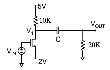
Problem 3 Assume the transistor is fabricated in a process with  $\mu C_{OX}=100 \mu A/V^2$ ,  $V_T = 0.75V$ ,  $\lambda = .01v^{-1}$ ,  $\gamma = 0$  and  $\phi = 0.6V$  and that the bulk (not shown) is connected to the source.
