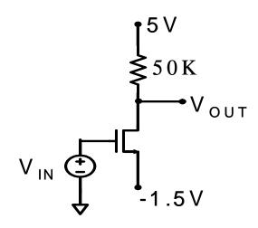
Problem 4 Assume the transistor is fabricated in a process with  $\mu C_{OX}=100 \mu A/V^2$ ,  $V_T = 0.75V$ ,  $\lambda = .01v^{-1}$ ,  $\gamma = 0$  and  $\phi = 0.6V$  and that the bulk (not shown) is connected to the source.
