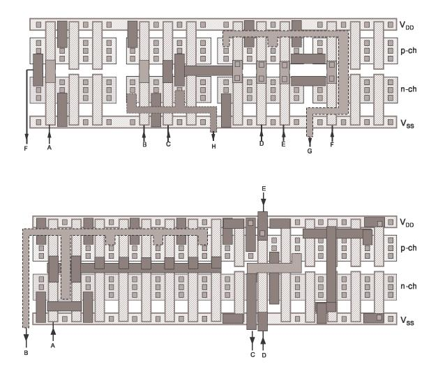
Problem 6 Design a 3input OR gate and a 2 input NAND gate in static CMOS. First size the devices for an overdrive of 1 and then size the devices for an overdrive of 4.
