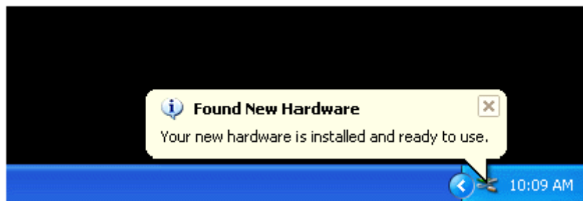
Figure A.14 Notification that the QIC is ready for use on a PC with Windows XP.
