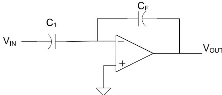
Figure 1 Voltage Amplifier with Capacitive Beta Feedback Network
