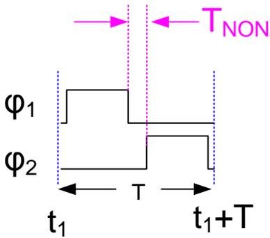
Figure 4 Non-overlapping Complimentary Clock Signals
