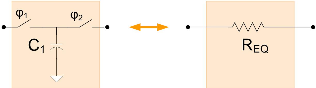
Figure 7 Equivalence of switched capacitor to a resistor for high clock frequencies
