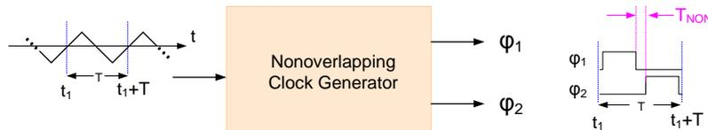
Part 2 Design and test a Switched Capacitor Amplifier that has a voltage gain of -20. Use either the MAX 326 or the MAX 364 analog switches. Use a 100KHz clock and the nonoverlapping
