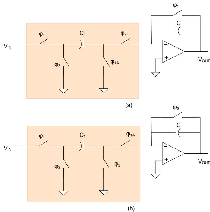
Figure 5 Stray Insensitive Switched Capacitor Amplifier a) noninverting, b) inverting
