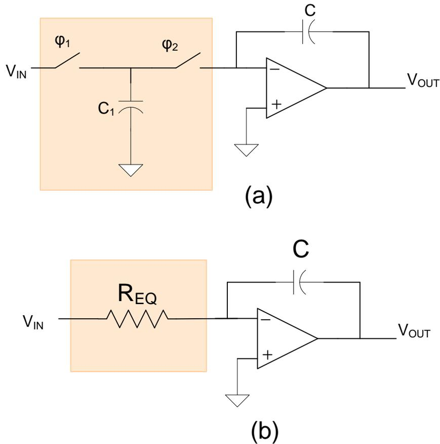
Figure 6 Integrators a) Switched-Capacitor Integrator b)RC Integrator
