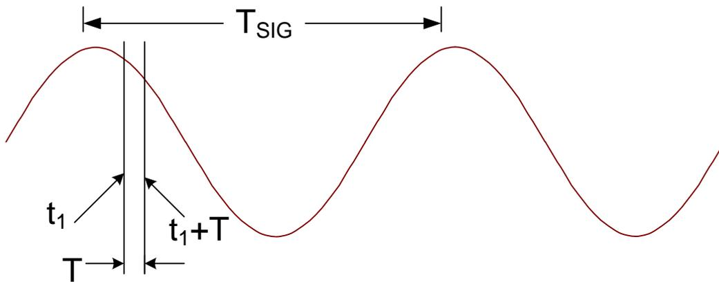
Figure 3 Timing of Switched Capacitor Clock and Input Signals
