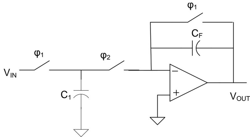
Figure 2 Basic Switched Capacitor Amplifier
