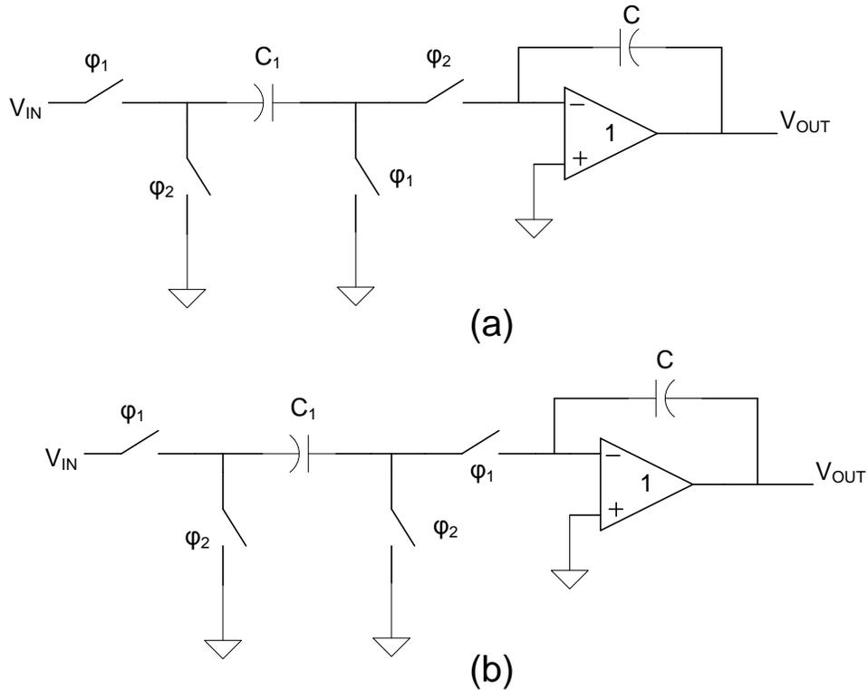
Figure 8 Stray Insensitive Switched Capacitor Integrators a) Noninverting b) Inverting
