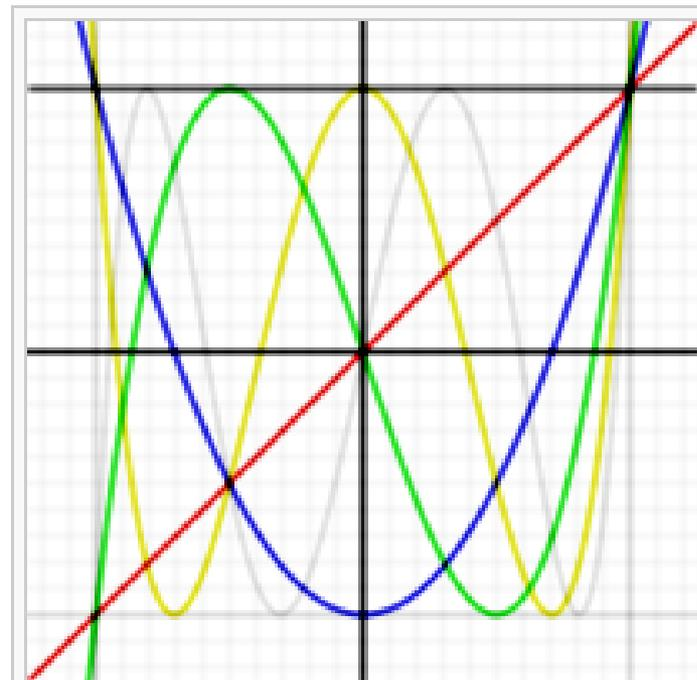
This image shows the first few Chebyshev polynomials of the first kind in the domain  $-1 \leq x \leq 1$ ,  $-1 \leq y \leq 1$ ; the flat  $T_0$ , and  $T_1$ ,  $T_2$ ,  $T_3$ ,  $T_4$  and  $T_5$ . Figure from Wikipedia
