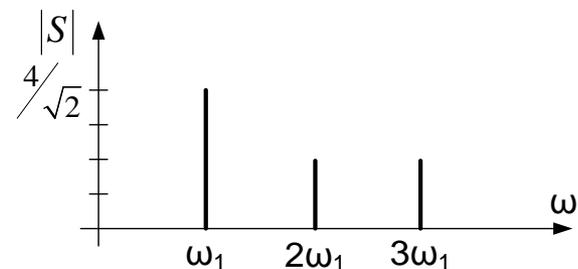
**Nonlinear distortion evidenced by presence of spectral components in output that are not in the input**
