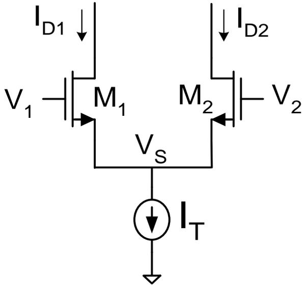
$$\frac{I_T}{2} = \frac{\mu C_{ox} W}{2L} (V_{EB})^2$$
