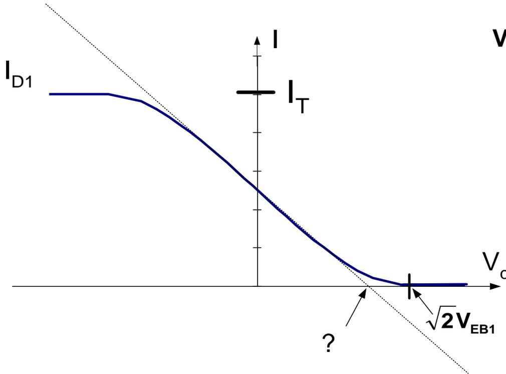
$$V_d = \sqrt{\frac{2L}{\mu C_{ox} W}} \left( \sqrt{I_T - I_{D1}} - \sqrt{I_{D1}} \right)$$
