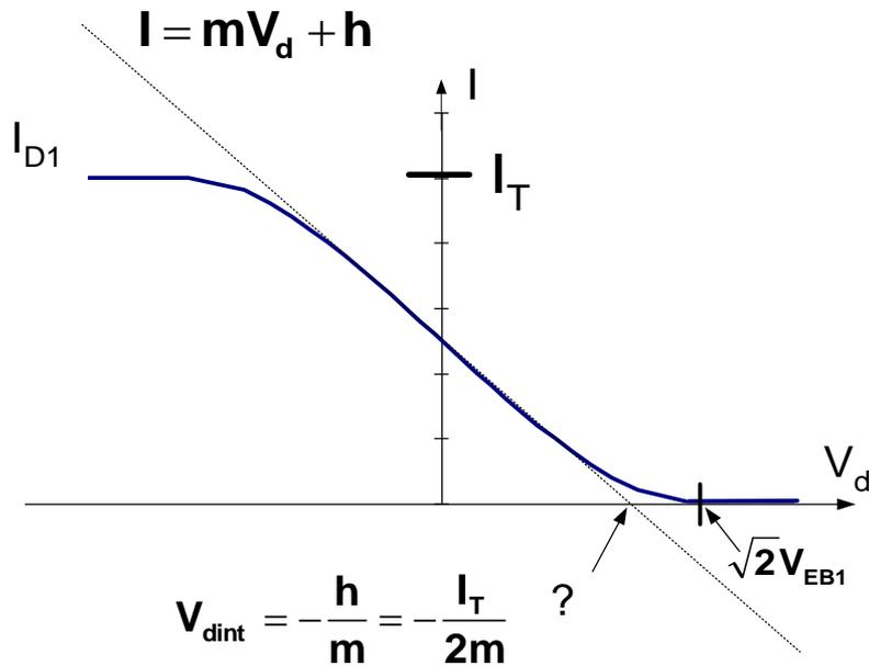
$$m = \left. \frac{\partial I_{D1}}{\partial V_d} \right|_{Q-pt}$$
