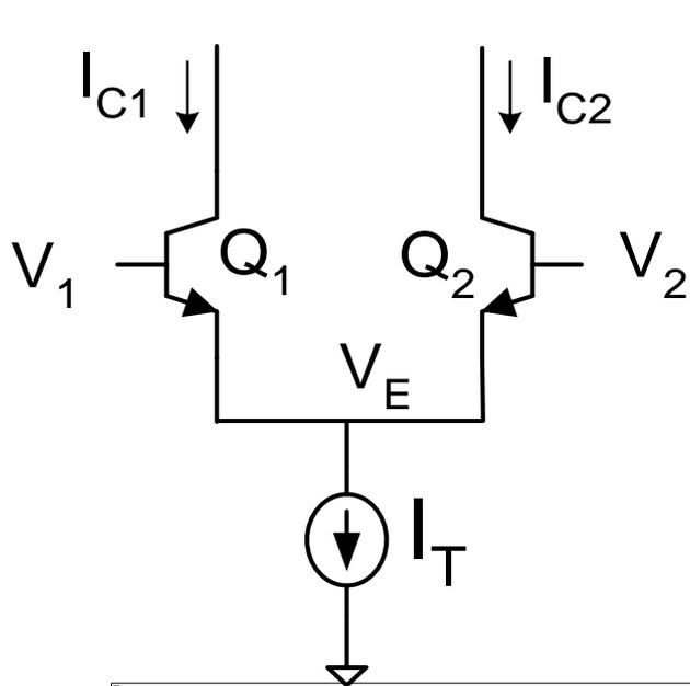
$$I_{C1} = J_S A_{E1} e^{\frac{V_1 - V_E}{V_t}}$$
