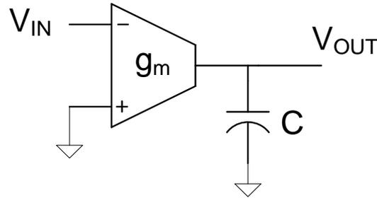
Transconductor-based filters depend directly on the  $g_m$  of the transconductor
