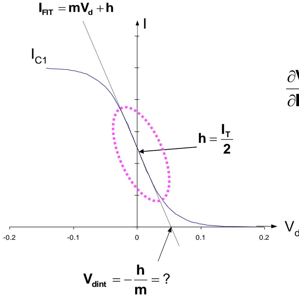
$$m = \left. \frac{\partial I_{C1}}{\partial V_d} \right|_{Q\text{-point}}$$
