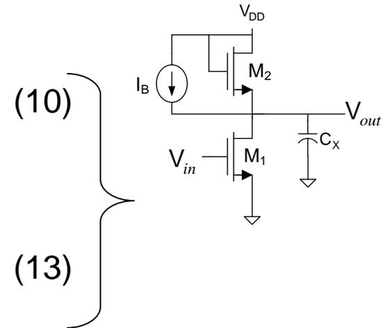
There is still one degree of freedom remaining. Can either pick  $W_1/L_1$  and solve for  $C_X$  or pick  $C_X$  and solve for  $W_1/L_1$ .
