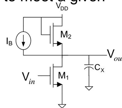
Still must obtain  $W_1/L_1$ ,  $V_{EB1}$ , and  $C_X$  from either of these equations
