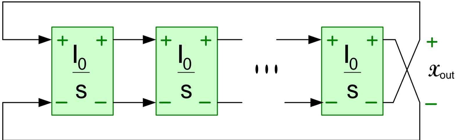
If fully differential or fully balanced, must have an odd number of crossings of outputs
