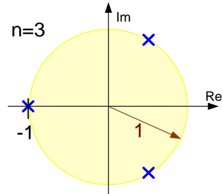
Roots are uniformly spaced on a unit circle
