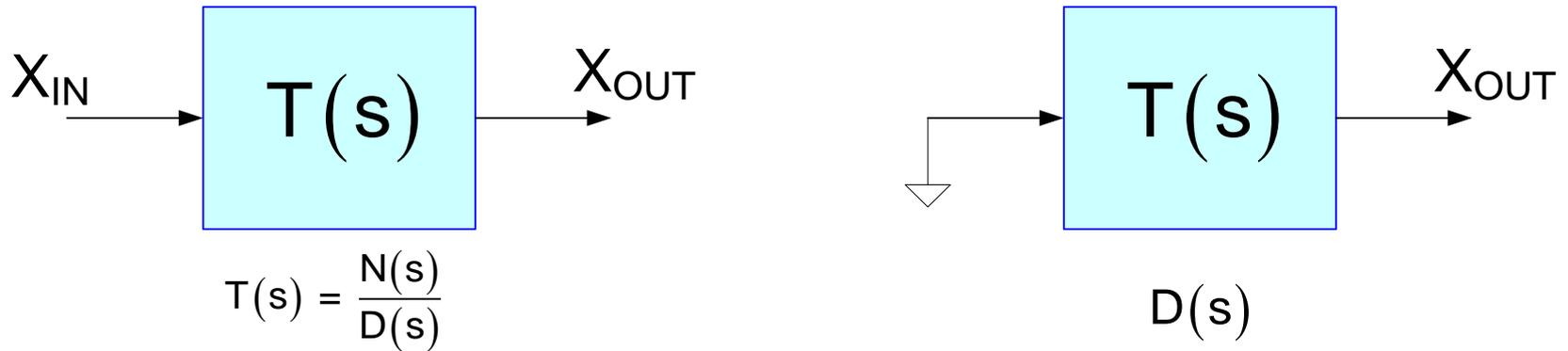
The “dead network” of any linear circuit is obtained by setting ALL independent sources to zero.
