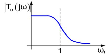
Frequency scaling by  $\omega_0$  (of transfer function)
