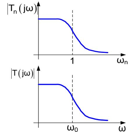
Frequency scaling / normalization does not change the shape of the transfer function, it only scales the frequency axis linearly
