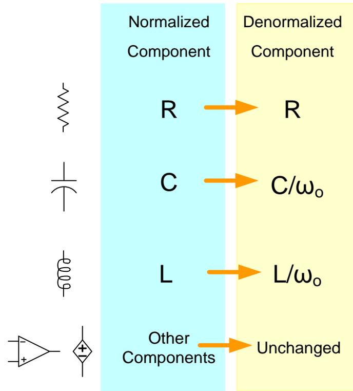
Component values of energy storage elements are scaled down by a factor of  $\omega_0$
