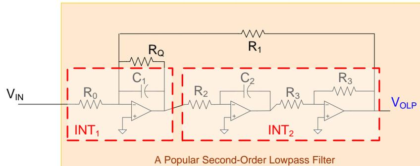
If  $C_1=C_2=C$  and  $R_1=R_2=R_0=R$ , this reduces to
