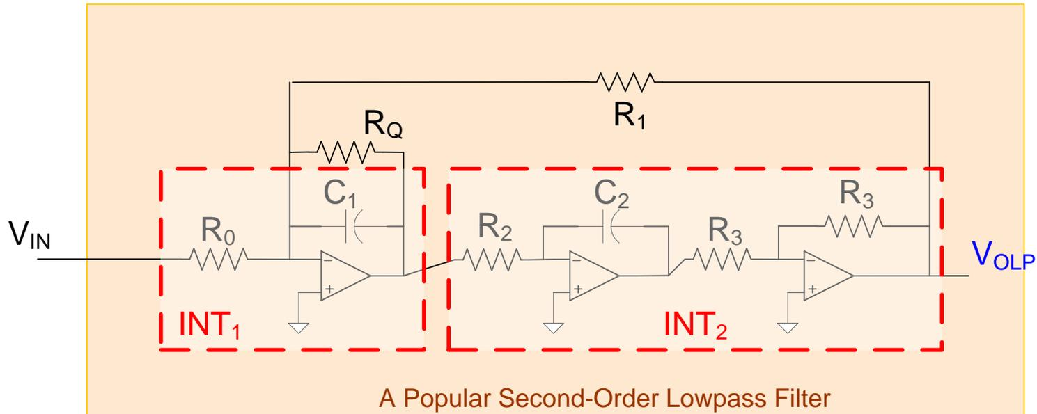
Example: Design a 2<sup>nd</sup> order lowpass Butterworth filter with 3dB passband attenuation, a dc gain of 5, and a 3dB band edge of 4KHz
