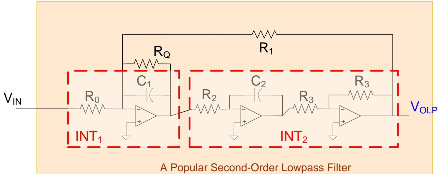
$$T(s) = \frac{1}{R_2 R_0 C_1 C_2} \frac{1}{s^2 + s \left( \frac{1}{R_Q C_1} \right) + \frac{1}{R_2 R_1 C_1 C_2}}$$
