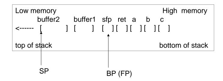
Offsets relative to BP are used as addresses within the function to access local variables and parameters.
