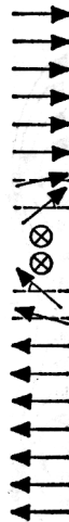
FIG. 7.3 Reversal of magnetization vectors in a Néel wall producing a short length of Bloch wall; the diagram also applies to a short length of Néel wall in a Bloch wall.
