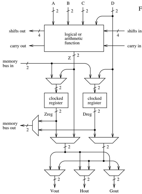
Figure 4: Simplified logic block schematic.
