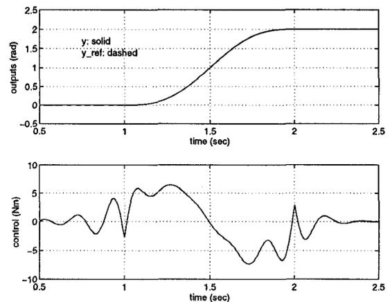
Figure 2: Simulation by Stable Inversion
