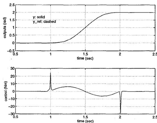
Figure 3: Simulation by input/output linearization
