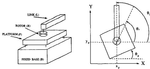
Figure 1: Flexible-joint robot on wobbly platform
