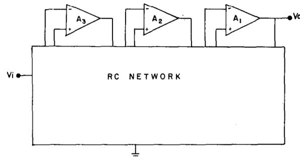
Fig. 1. General three op amp active filter.
