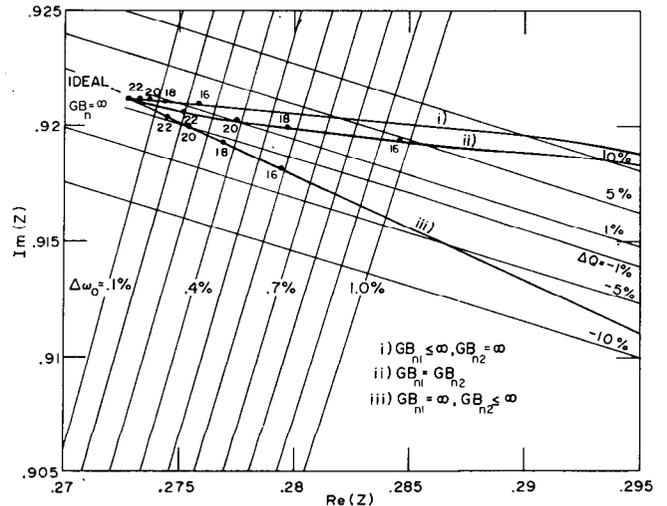
Fig. 9. Root locus of Biquad 2 for different values of  $GB_n$ 's.  $GB_i = GB_{ni}$ ,  $i = 1, 2$ .
