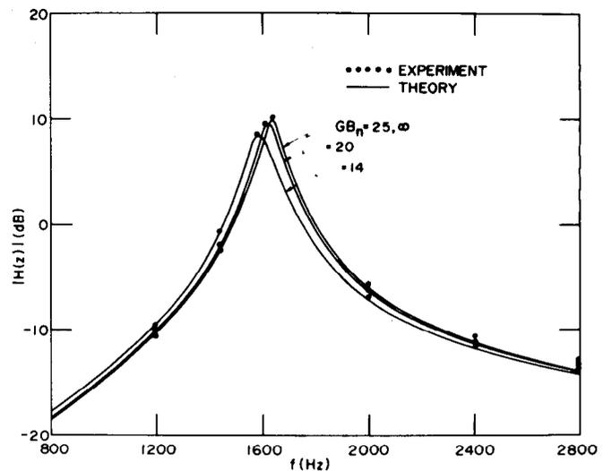
Fig. 5. Theoretical and experimental frequency response of Biquad 1.
