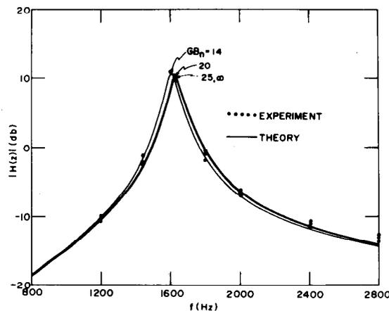
Fig. 6. Theoretical and experimental frequency response of Biquad 2.
