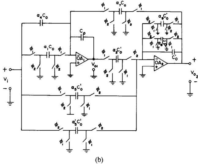
Fig. 2. Generation of Biquad 1. a) Flow diagram. b) SC implementation.
