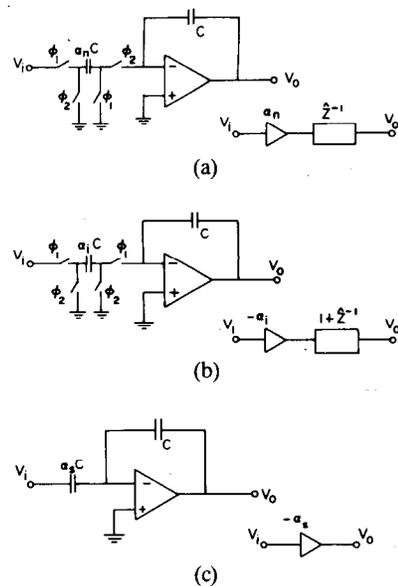
Fig. 1. Basic cells. (a) Noninverting integrator. (b) Inverting integrator. (c) Inverting amplifier.
