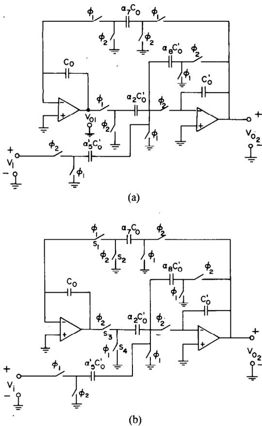
Fig. 4. SC Bandpass minimum switch configurations. (a) Biquad 1. (b) Biquad 2.
