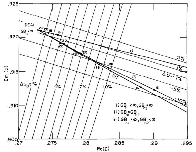
Fig. 8. Root locus of Biquad 1 for different values of  $GB_n$ 's.  $GB_i = GB_{ni}$ ,  $i = 1, 2$ .
