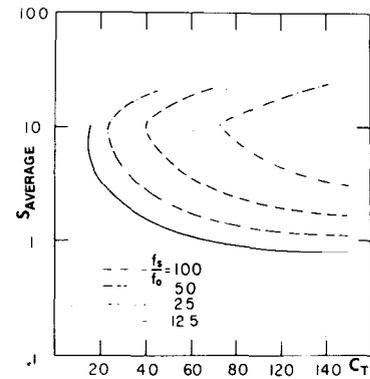
Fig. 3. Average  $Q$  sensitivity versus total capacitance for a fixed  $Q=10$ , and different  $f_0/f_s$  values.
