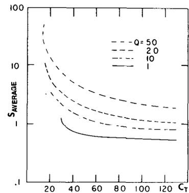
Fig. 4. Average  $Q$  sensitivity versus total capacitance for a fixed  $f_0/f_s = 1/10$ , and different  $Q$  values.
