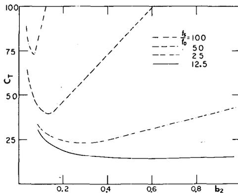
Fig. 2. Total capacitance versus the capacitor ratio  $b_2$  for a fixed  $Q=10$ , and different  $f_0/f_s$  values.
