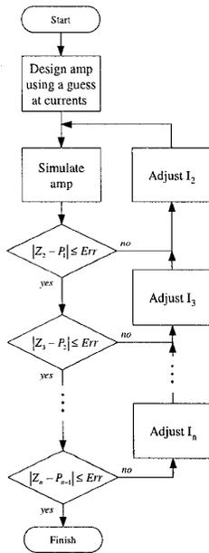
Figure 7: Design procedure used to optimize the amplifier response
