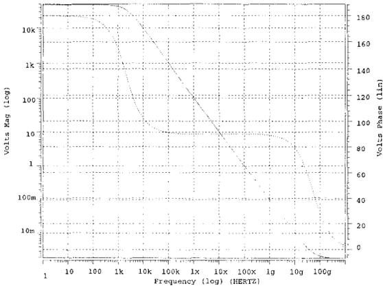
Figure 8: Simulated open loop response of the multipath compensated amplifier
