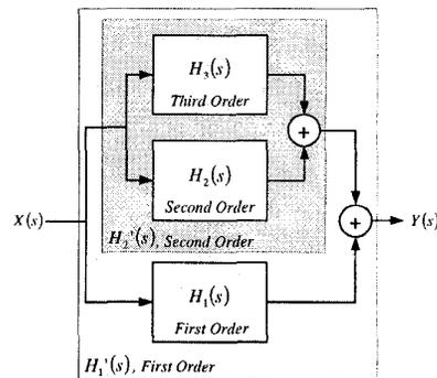
Figure 2: Design of three stage amplifier using multipath compensation
