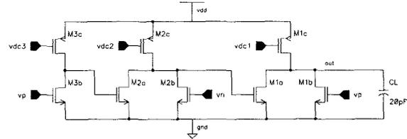
Figure 6: Circuit that was simulated to demonstrate the validity of the multipath compensation concept
