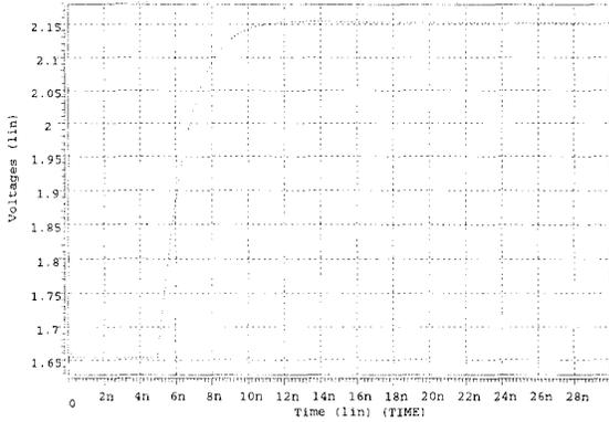
Figure 9: Simulated unity-gain step response of the multipath compensated amplifier
