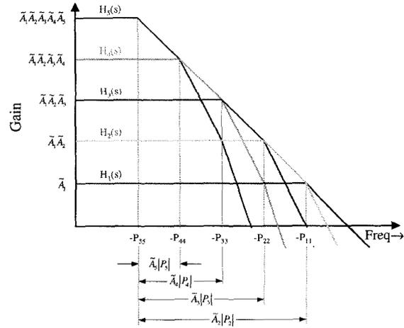
Figure 5: Required pole locations in terms of  $\tilde{A}_i$ 's for a five stage multipath compensated amplifier
