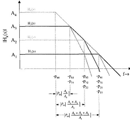
Figure 3: Approximate magnitude plots of the constituent systems' required transfer functions
