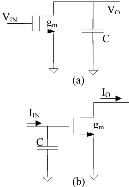
Fig. 5 Inverting Lossless High-Speed Integrators a) Voltage-mode, b) Current-mode
