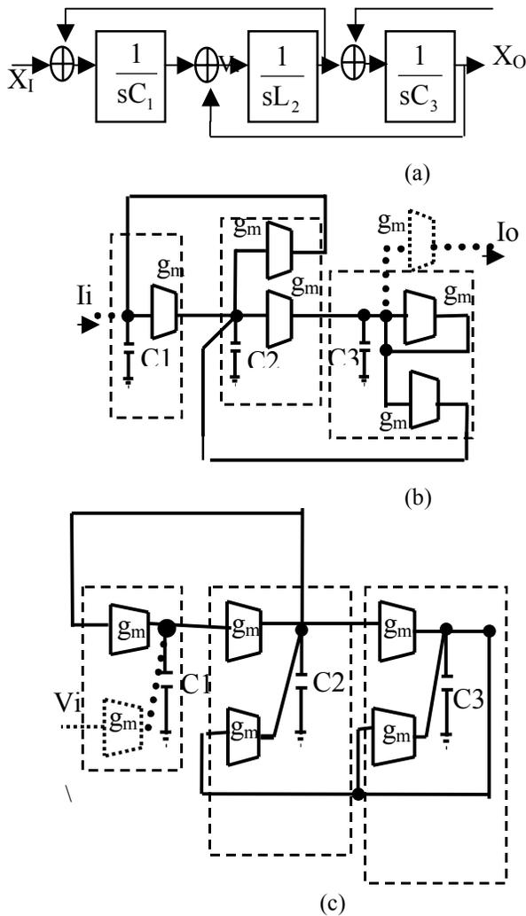
Fig. 9 Leapfrog Block Implementation a) Block Diagram, b) Current-Mode Implementation, c) Voltage-Mode Implementation
