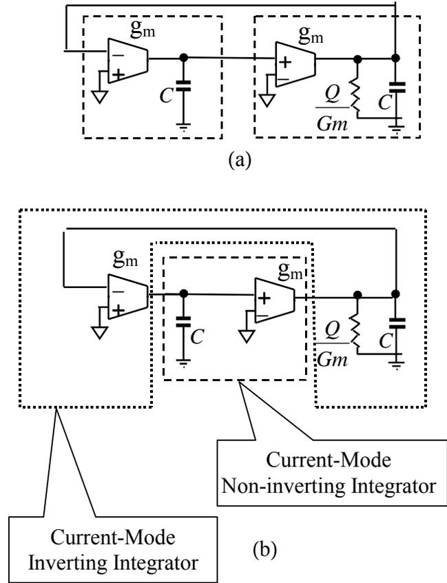
Fig. 8 Two representations of the voltage-mode two-integrator loop a) standard voltage-mode implementation, b) current-mode equivalent
