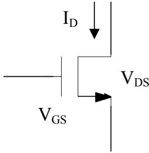
Fig. 2 A simple MOS transistor – Current-mode or Voltage-mode?
