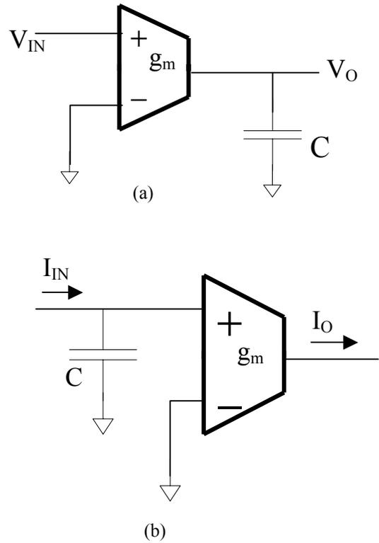
Fig. 3 Lossless Non-inverting Gm-C Integrators
