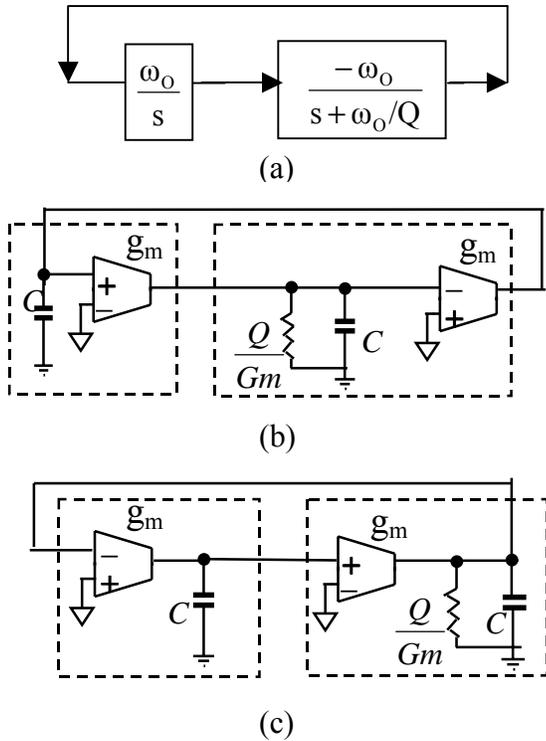
Fig.7 A two-integrator loop biquad a) block diagram b) current-mode implementation c) voltage-mode implementation
