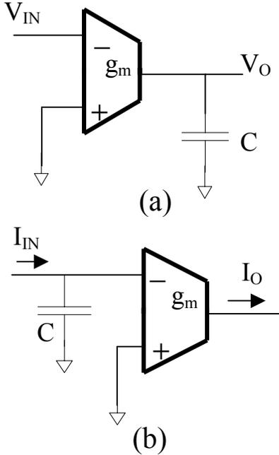
Fig. 4 Inverting Lossless Gm-C Integrators a) Voltage-mode, b) Current-mode
