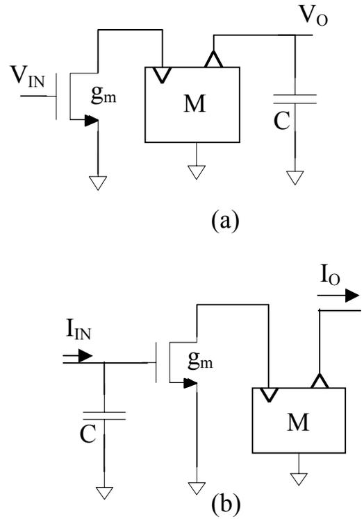
Fig. 6 Non-inverting Lossless High-Gain Integrators a) Voltage-mode, b) Current-mode
