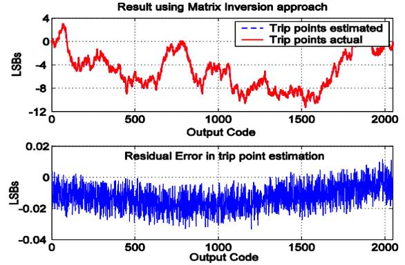
Figure.2. Introduced and Estimated trip point errors
