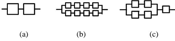
Fig. 1: Three different approaches to implement the same resistor
