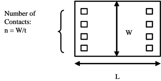
Fig. 3: A symbolic layout of rectangular resistor
