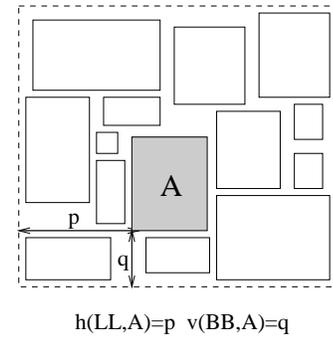
Fig. 6. Examples of preplace constraint.
