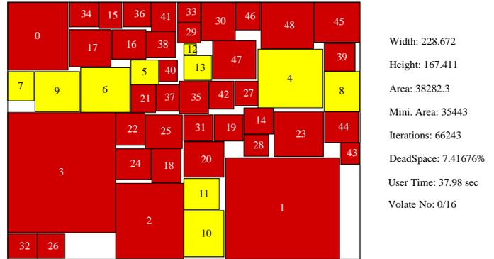
Fig. 14. Modules 4, 5, 6, 7, 8 and 9 almost align horizontally. Modules 10, 11, 12 and 13 align vertically.
