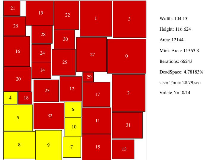
Fig. 11. Modules 4, 5, 6, 7, 8, 9 and 10 cluster at the lower left corner of the chip.
