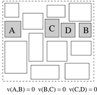
Fig. 4. Examples of alignment constraint.
