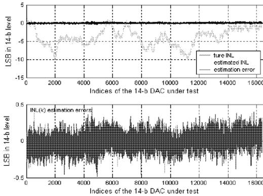
Figure 7. INL(k) estimation error with P=16 and 5-bit dithering DAC, 14 bits DAC under test
