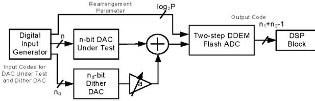
Figure 4. Block diagram of the proposed BIST scheme
