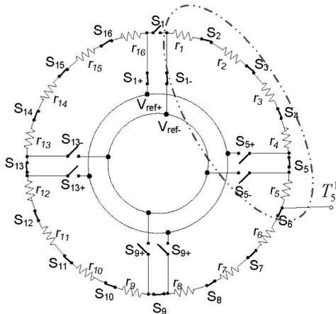
Figure 2. Resistor loop of a 4-bit DDEM flash ADC with  $P = 4$
