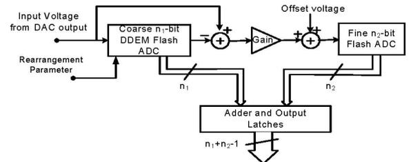
Figure 3. Block diagram of the two-step DDEM flash ADC
