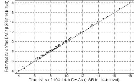
Figure 8. Estimated INLs vs true INLs of 100 14-bit DACs tested by 100 DDEM ADC transition points
