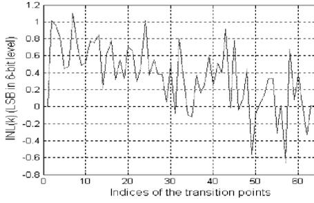
Figure 6. Linearity of the original coarse stage flash ADC
