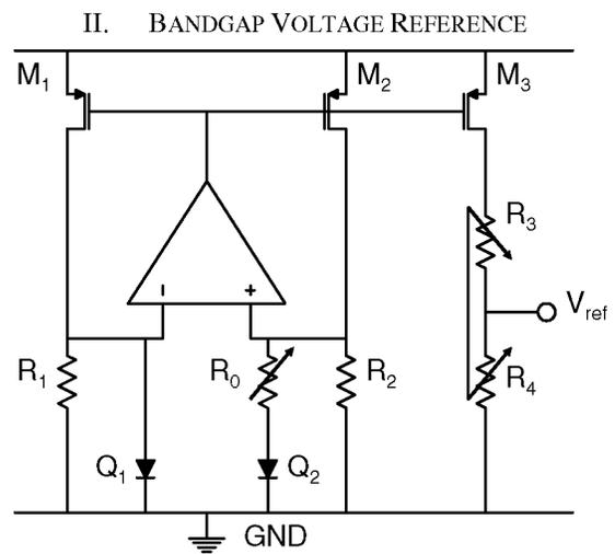
Figure 1. Schematic of the multi-segment bandgap reference.
