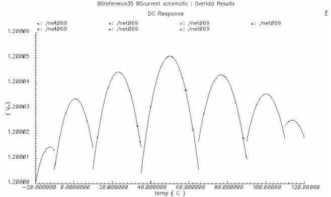
Figure 6. Self-calibrated multi-segment bandgap voltage curve.
