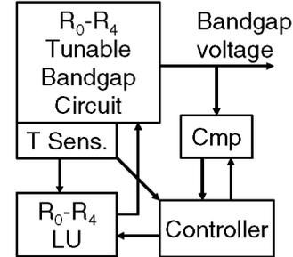
Figure 3. Block diagram of the bandgap circuit with self-calibration.
