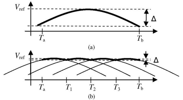
Figure 2. Conceptual depiction of (a) Single-inflection point bandgap curve and (b) Multi-segment bandgap curve.
