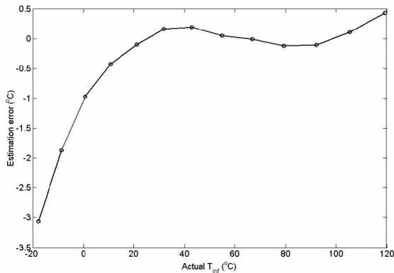
Figure 5. Estimation error in  $T_{inf}$ - $R_0$  relationship.
