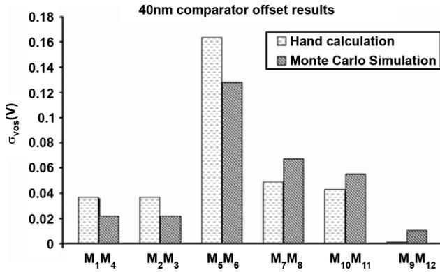
Fig. 4. Comparison between analytical results and Monte Carlo simulation for each pair in a 40-nm comparator.
