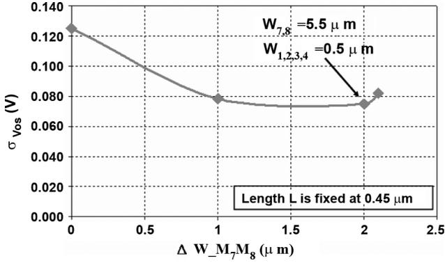
Fig. 7. Random offset versus  $\Delta W$  of matching critical pair  $M_7M_8$ .
