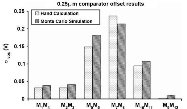
Fig. 3. Comparison between analytical results and Monte Carlo simulation for each pair in a 0.25- $\mu\text{m}$  comparator.
