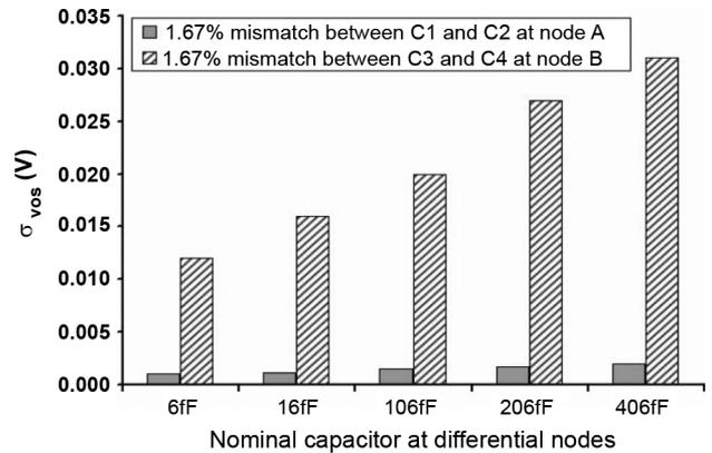
Fig. 6. Dynamic offsets from  $C_1$  &  $C_2$  and  $C_3$  &  $C_4$  mismatch.
