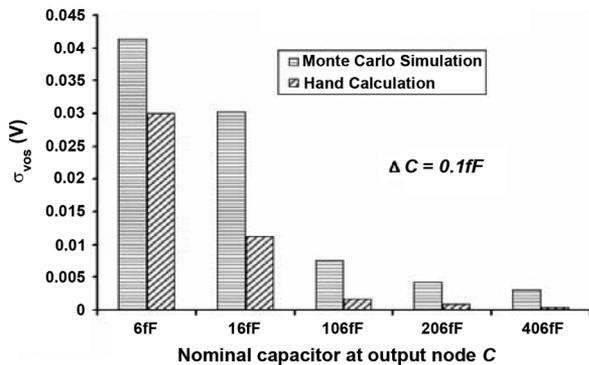
Fig. 5. Comparison of dynamic offset voltages due to  $C_{5,6}$  mismatch derived by analytical model and Monte Carlo simulation.
