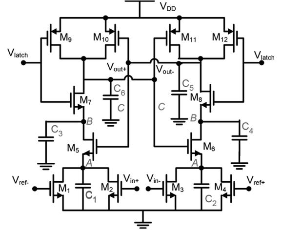
Fig. 2. “Lewis-Gray” structure with internal parasitic capacitors.
