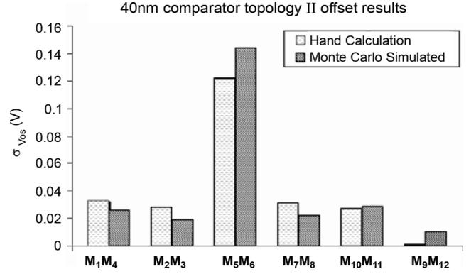
Fig. 10. Comparison between analytical results and Monte Carlo simulation for each pair in 40 nm comparator in Fig. 9.
